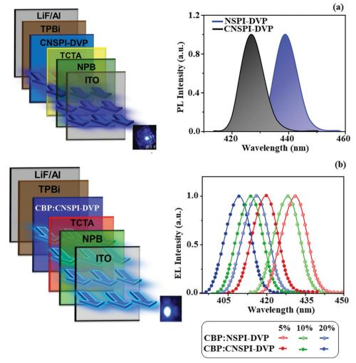
Fig. 11 Device configuration with EL spectra: (a) non-doped and (b) doped devices.
