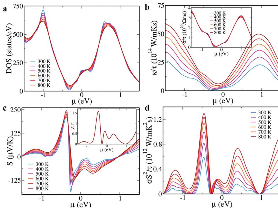
Fig. 3 (a) DOS; (b) thermal conductivity (inset: electrical conductivity); (c) Seebeck co-efficient (inset:  $ZT$  at 800 K) and (d) power factor of  $\text{Sn}_{10}\text{Pb}_5\text{BiTe}_{16}$  as a function of chemical potential ( $\mu$ ) at various temperatures. The conductivity and power factor values are reported by scaling it with  $\tau$ .
