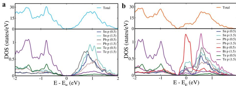
Fig. 2 pDOS of (a)  $\text{Sn}_{11}\text{Pb}_5\text{Te}_{16}$ ; and (b)  $\text{Sn}_{10}\text{Pb}_5\text{BiTe}_{16}$ . The energy levels are shifted with respect to the Fermi level of the configurations, which is set to zero.
