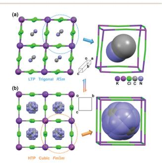
Fig. 2 Crystal structures of 1 at (a) LTP (293 K) and (b) HTP (373 K). The MA cations display a highly disordered state at HTP. Hydrogen atoms are omitted for clarity.
