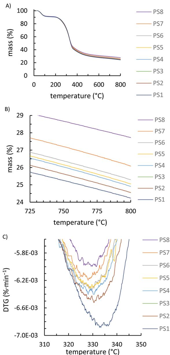
Fig. 3 Thermogravimetric analysis of **PS-X** fractions from 25–800 °C (A), from 725–800 °C to emphasize the difference in residual mass (B), and the derivative TGA (DTG) curve over the primary decomposition step, emphasizing the more rapid and lower-temperature decomposition with smaller particle size (C). Note that **PS-2** and **PS-3** are coincident.
