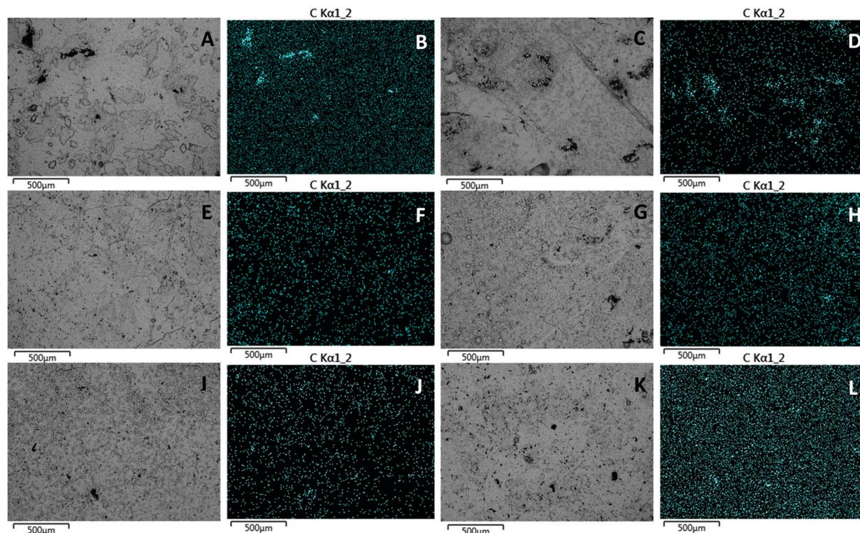
Fig. 6 SEM-EDX images of **PSS-X** showing the EM image (black and white: A, C, E, G, I and K) and the carbon element mapping (blue images: B, D, F, H, J and L) for **PSS-3** (A and B), **PSS-4** (C and D), **PSS-5** (E and F), **PSS-6** (G and H), **PSS-7** (I and J), and **PSS-8** (K and L).
