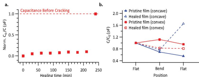
Fig. 4 (a) Evolution of the capacitance during the healing process measured for an area of 1.0 cm<sup>2</sup>. (b) Static capacitance measurement of pristine and healed films in both concave and convex positions.
