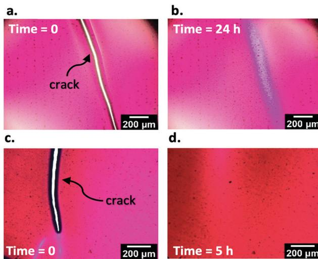
Fig. 2 Self-healing of polymer **1** in thin films visualized by optical microscopy (a) before and (b) after 24 hours of healing at room temperature, and (c) before and (d) after 5 hours of healing at human body temperature ( $37\text{ }^\circ\text{C}$ ).
