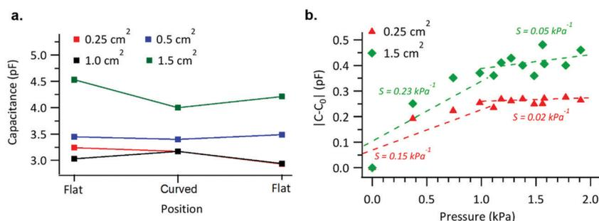
Fig. 3 (a) Static measurement of capacitance as a function of curvature for flat ( $1/r \approx 0$ ) and curved ( $1/r = 0.17$ ) positions for different capacitor areas, and (b) representative capacitance variation as a function of applied pressure, for capacitors with 0.25 (red) and 1.5 cm<sup>2</sup> (green) electrode area.
