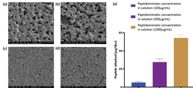
Fig. 5 (a) and (c) Scanning electron micrographs of HA discs incubated in water for 24 h and (b) and (d) incubated in 1000 μg mL<sup>-1</sup> peptidomimetic solution for 24 h. (e) Quantification of peptidomimetic attachment on HA discs corresponding to three different concentrations of peptidomimetic loading solution. *n* = 3.
