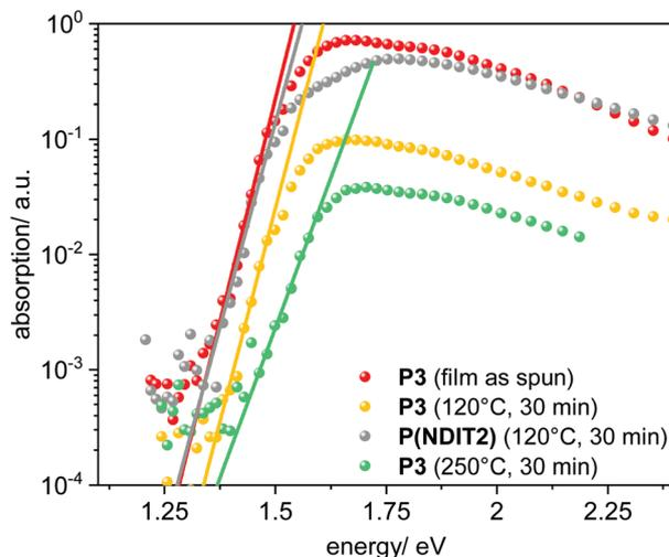
Fig. 6 Comparison between the absorption of P3 ( $M_n = 61 \text{ kg mol}^{-1}$ ) and P(NDIT2) ( $M_n = 62 \text{ kg mol}^{-1}$ ) thin films in dependence of the annealing temperature; measured by photothermal deflection spectroscopy. The solid line displays the corresponding exponential fits for extraction of the Urbach energy  $U_{\text{E}}$ . Films were spin-coated (1000 rpm, 60 s) from *o*-DCB solutions.
