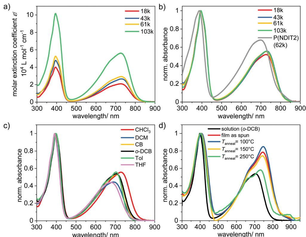
Fig. 2 Molar extinction coefficient (a) and normalized (b) UV-vis spectra of P(NDI-IDT) of different MW ( $M_n$  in  $\text{g mol}^{-1}$ ) in chloroform solution at room temperature. Solvent dependent (c) and film (d) UV-vis spectra of **P3** ( $M_n = 61 \text{ kg mol}^{-1}$ ).
