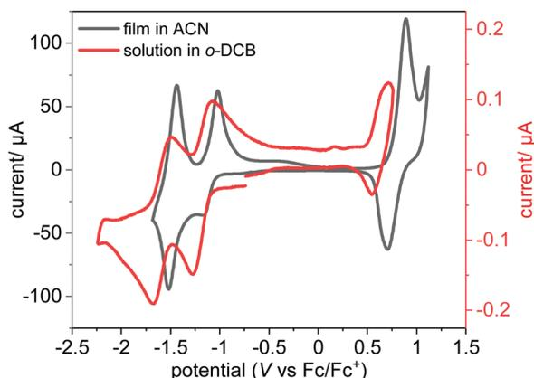
Fig. 3 Cyclic voltammograms of P(NDI-IDT) as film deposited on an ITO substrate in a  $0.1 \text{ M NBu}_4\text{PF}_6$  acetonitrile solution (black) and in a  $0.1 \text{ M NBu}_4\text{PF}_6$  *o*-DCB solution (red) at a scan rate of  $50 \text{ mV s}^{-1}$ .
