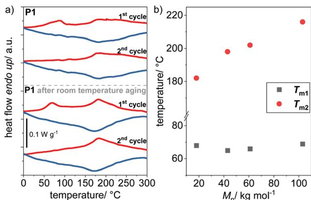
Fig. 4 (a) DSC curves of **P1** ( $M_n = 18 \text{ kg mol}^{-1}$ ). First and second cycles were measured under  $N_2$  with  $10 \text{ K min}^{-1}$  before and with  $20 \text{ K min}^{-1}$  after room temperature aging; (b) side chain  $T_{m1}$  and main chain  $T_{m2}$  melting transitions in dependence of  $M_w$ .
