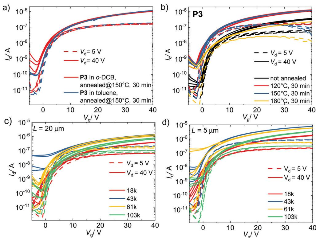
Fig. 5 Optimization of OFET devices. Effect of solvent for spin coating (a) and annealing temperature for **P3** (b). Transfer curves of optimized devices as a function of MW ( $\text{g mol}^{-1}$ ) and channel length (c and d).
