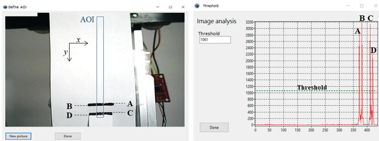
Fig. 2 Video extensometer menu with AOI (left) and defined threshold (green dashed line) for the resulting red trace (right). Graph: averaged difference values as a function of vertical ( $y$ ) pixel number in AOI.
