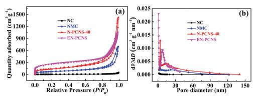
Fig. 4 (a) N<sub>2</sub> adsorption/desorption isothermal curves and (b) pore size distribution curves of the NC, NMC, N-PCNS-40, and EN-PCNS samples.
