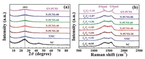
Fig. 2 (a) XRD patterns and (b) Raman spectra of NC, NMC, N-PCNS-m and EN-PCNS.
