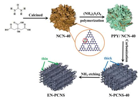
Fig. 1 The synthetic scheme of EN-PCNS.
