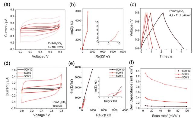
Fig. 5 Electrochemical characterization of IDE 500/10 pyrolyzed at 900 °C (CV-curves (a), Nyquist plot (b), GCD-curves (c)) and of the three different structures (CV-curves (d), Nyquist plot (e), device Capacitances (f))
