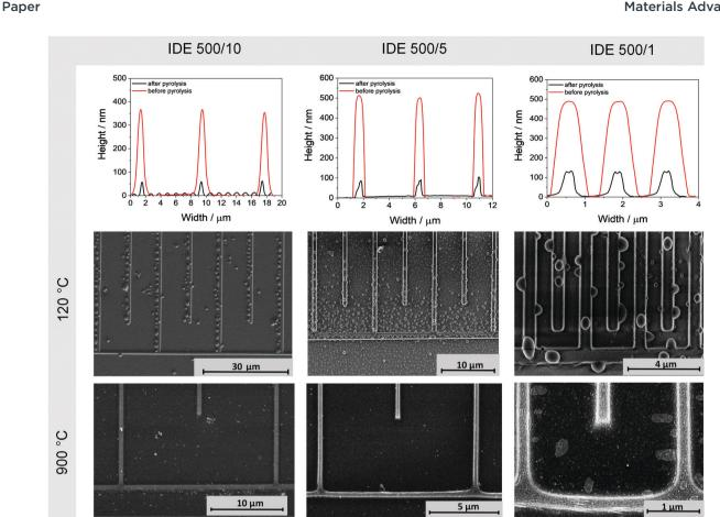
Fig. 3 Height profiles (after printing red lines (polymer), after pyrolysis black lines (carbon)) of the different structures and SEM images of the three different structures after printing at 120 °C and after carbonization at 900 °C
