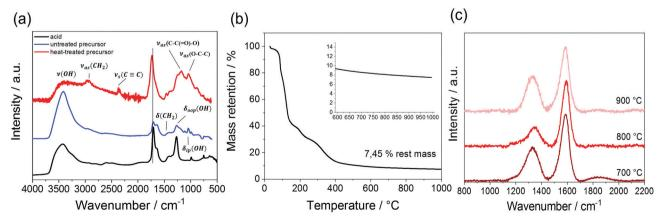
Fig. 2 IR-spectra of the pure acid (black line), the untreated (blue line) and treated precursor (red line) (a), thermal analysis (b), Raman-spectra of the precursor powders carbonized at 700 °C, 800 °C and 900 °C in Ar-atmosphere (c).
