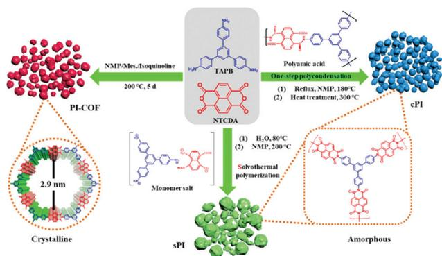
Scheme 1 Schematic of synthesis processes for different-type polyimides.
