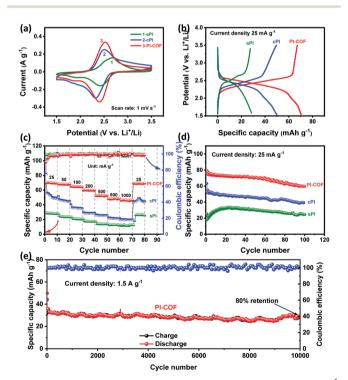
Fig. 4 (a) CV curves of sPI, cPI and PI-COF at a scan rate of 1 mV s $^{-1}$ , (b) discharge—charge profiles of the three samples at 25 mA  $g^{-1}$ , (c) rate capability and (d) cycling performance at 25 mA  $g^{-1}$  of sPI, cPI, and PI-COF. (e) Long-term cyclability of PI-COF at 1.5 A  $g^{-1}$ .
