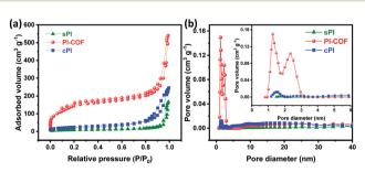
Fig. 3 (a) Nitrogen adsorption—desorption isotherms, and (b) pore size distributions of sPI, cPI, and PI-COF.
