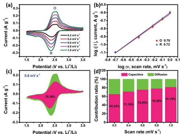
Fig. 5 (a) CVs of PI-COF at different scan rates from 0.2 to  $1 \text{ mV s}^{-1}$ . (b)  $\log i$  vs  $\log \nu$  plots. (c) Capacitive and diffusion-controlled contribution to the charge storage of PI-COF ( $0.8 \text{ mV s}^{-1}$ ) and (d) contribution ratios of capacitive- and diffusion-controlled capacity for PI-COF at different scan rates.
