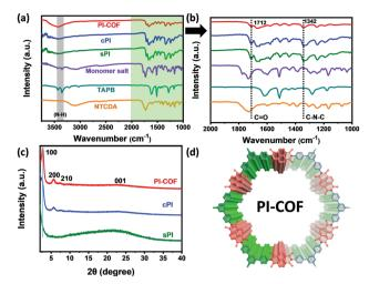
Fig. 1 (a) FT-IR spectra of TAPB, NTCDA, monomer salt, and PI products. (b) Zooming in the characteristic region of 1000–2000 cm<sup>-1</sup>. (c) XRD patterns of sPI, cPI, and PI-COF. (d) HR-TEM image of PI-COF.
