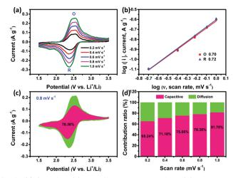
Fig. 5 (a) CVs of PI-COF at different scan rates from 0.2 to 1 mV  $\rm s^{-1}$ . (b)  $\log i \ vs \log \nu$  plots. (c) Capacitive and diffusion-controlled contribution to the charge storage of PI-COF (0.8 mV  $\ensuremath{\text{s}^{-1}}\xspace$ ) and (d) contribution ratios of capacitive- and diffusion-controlled capacity for PI-COF at different scan
