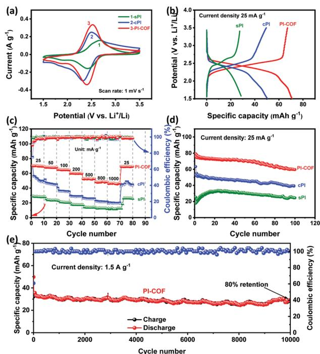
Fig. 4 (a) CV curves of sPI, cPI and PI-COF at a scan rate of  $1 \text{ mV s}^{-1}$ , (b) discharge–charge profiles of the three samples at  $25 \text{ mA g}^{-1}$ , (c) rate capability and (d) cycling performance at  $25 \text{ mA g}^{-1}$  of sPI, cPI, and PI-COF. (e) Long-term cyclability of PI-COF at  $1.5 \text{ A g}^{-1}$ .
