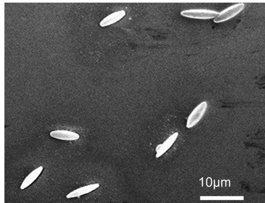
Fig. 3 SEM image of stretched ellipsoidal polystyrene colloids.
