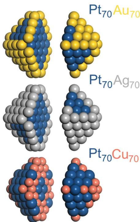
Fig. 1 Chemical orderings of ca. 1.4 nm large 140-atomic truncated-octahedral fcc nanoparticles Pt<sub>70</sub>Au<sub>70</sub>, Pt<sub>70</sub>Ag<sub>70</sub>, and Pt<sub>70</sub>Cu<sub>70</sub> with the lowest DFT energies. Particles images are split in two parts for better visualization. Pt – blue, Au – yellow, Ag – gray, Cu – red-brown.
