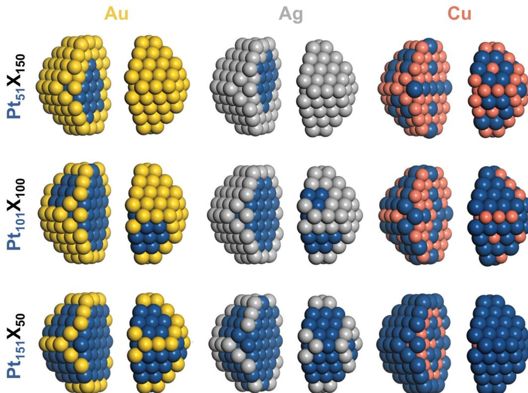
Fig. 2 Chemical orderings of 17–18 nm large 201-atomic truncated-octahedral fcc nanoparticles of the compositions Pt:X (X = Au, Ag, Cu):1:3 – Pt<sub>51</sub>X<sub>150</sub>, 1:1 – Pt<sub>101</sub>X<sub>100</sub>, 3:1 – Pt<sub>151</sub>X<sub>50</sub> with the lowest DFT energies. Particles images are split in two parts for better visualization. Colors of atoms as in Fig. 1.
