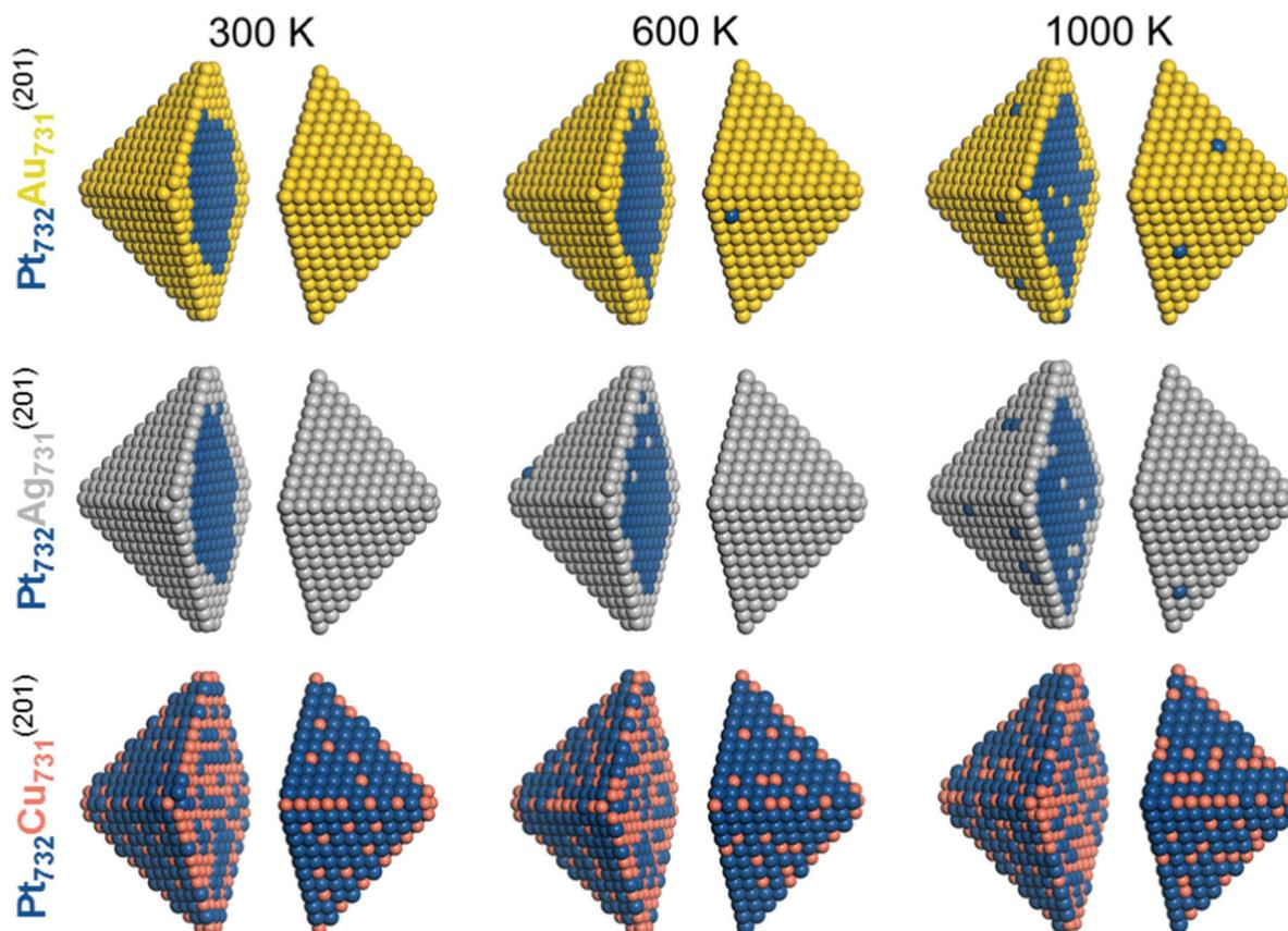
**Fig. 5** Equilibrium chemical orderings of  $\text{Pt}_{732}\text{Au}_{731}$ ,  $\text{Pt}_{732}\text{Ag}_{731}$ , and  $\text{Pt}_{732}\text{Cu}_{731}$  nanoparticles at temperatures 300 K, 600 K and 1000 K calculated using eqn (1) for the corresponding  $\text{Pt}_{101}\text{Au}_{100}$ ,  $\text{Pt}_{101}\text{Ag}_{100}$ , and  $\text{Pt}_{101}\text{Cu}_{100}$  particles. Colors of atoms are as in Fig. 1.
