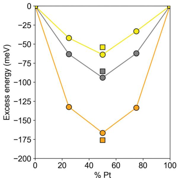
Fig. 3 DFT excess energies  $E_{\text{exc}}$  per atom (see eqn (2)) circles – of  $\text{Pt}_{201-n}\text{X}_n$  ( $X = \text{Au}, \text{Ag}, \text{Cu}; n = 50, 100, 150$ ) nanoparticles and squares – of  $\text{Pt}_{70}\text{X}_{70}$  nanoparticles. Pt–Au – yellow, Pt–Ag – gray, Pt–Cu – orange.
