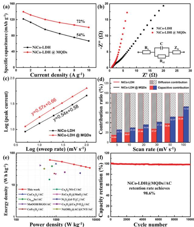
Fig. 4 (a) Specific capacities at different current densities and (b) Nyquist plots of Ni-Co LDH and Ni-Co LDH@MQDs. (c) Plots of  $\log(i)$  versus  $\log(\nu)$  of the samples. (d) The capacitive- and diffusion-controlled processes for Ni-Co LDH@MQDs at different scan rates. (e) Ragone plots. (f) Cycling performance of Ni-Co LDH@MQDs//AC at a current density of  $6\text{ A g}^{-1}$ .
