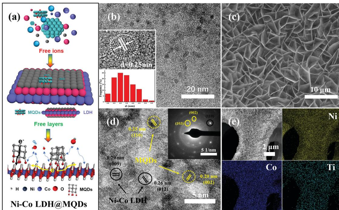
Fig. 2 (a) Schematic illustration of the bonding process. (b) HRTEM images with size distribution of MQDs. (c) SEM image of Ni-Co LDH@MQDs. (d) HRTEM images of Ni-Co LDH@MQDs (Inset: Diffraction and fringe pattern). (e) The uniform distribution of Ni, Co and Ti of Ni-Co LDH@MQDs.
