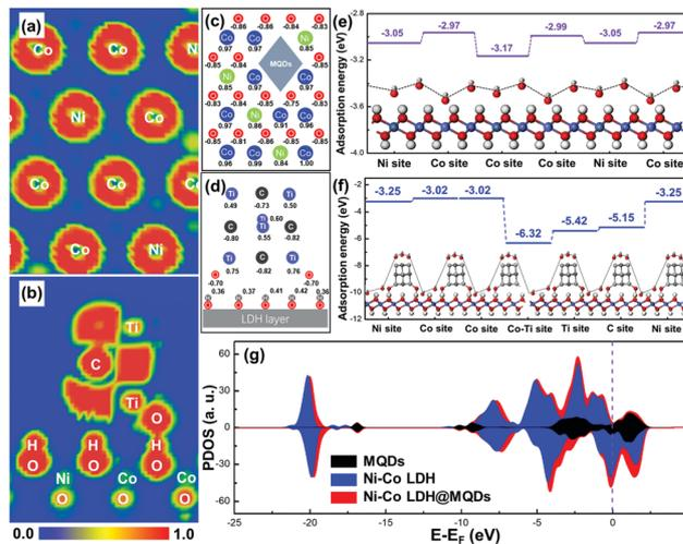
Fig. 1 ELF mappings of (a) LDH and (b) MQDs in Ni–Co LDH@MQDs. Calculated charge of surface atoms of (c) LDH and (d) MQDs in Ni–Co LDH@MQDs. Calculated adsorption energies using hydroxide ( $\text{OH}^-$ ) as an example for (e) Ni–Co LDH model and (f) Ni–Co LDH@MQDs. (g) Comparative DOS plots of MQDs, Ni–Co LDH and Ni–Co LDH@MQDs.
