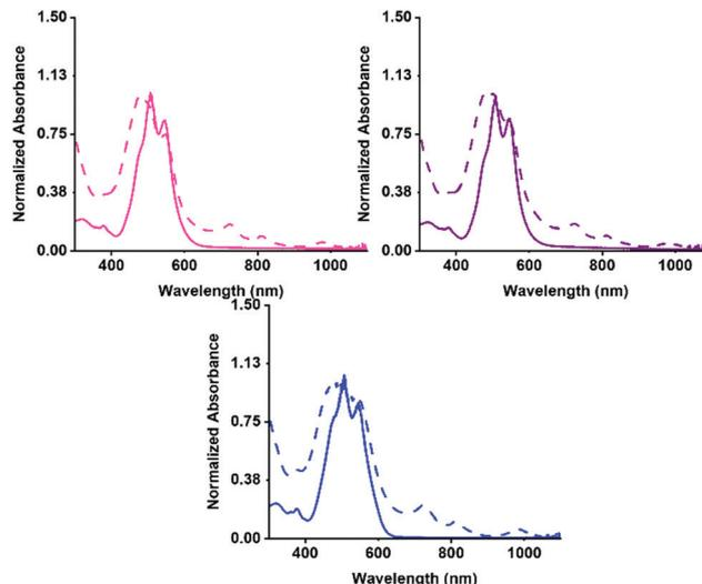
Fig. 2 UV-vis absorption spectra of **PBI-L** (solid pink), **PBI-I** (solid purple), **PBI-V** (solid blue) as at pH 7 and 10 mg mL<sup>-1</sup> solutions. UV-Vis absorption spectra of after being irradiated for 5 minutes using a 365 nm LED light for **PBI-L** (dashed pink), **PBI-I** (dashed purple), **PBI-V** (dashed blue).
