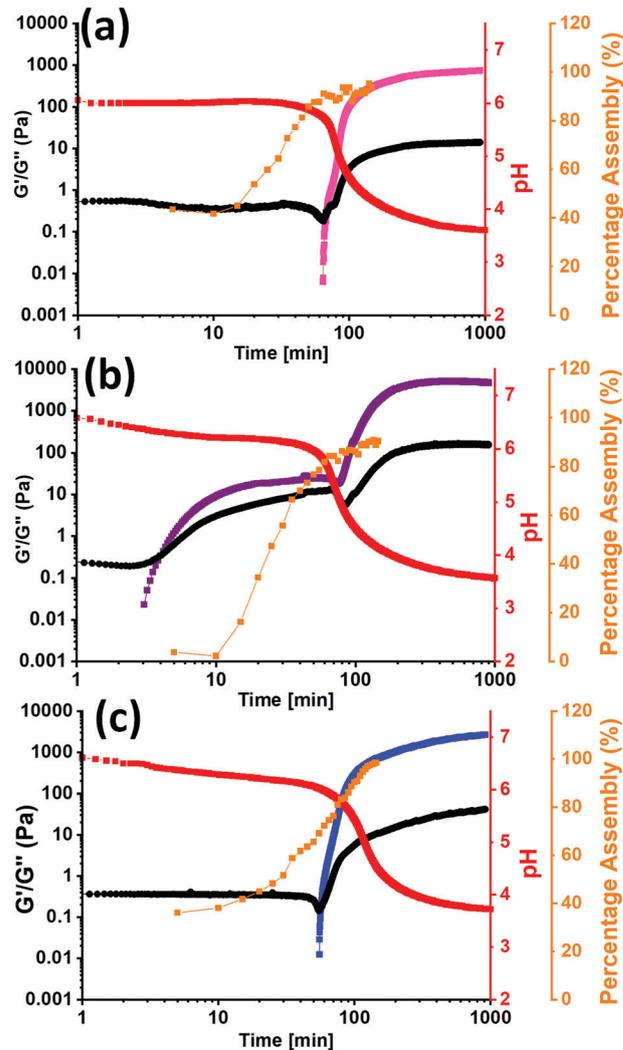
Fig. 4 Development of  $G'$  (pink, purple, blue data) and  $G''$  (black data) over time during the gelation of (a) **PBI-L** (pink), (b) **PBI-I** (purple) and (c) **PBI-V** (blue) at a strain of 0.5% and a frequency of  $10 \text{ rad s}^{-1}$ , compared to the change in pH (red data) over time and the change in percent assembled (orange data) over time calculated from the change in <sup>1</sup>H-NMR.
