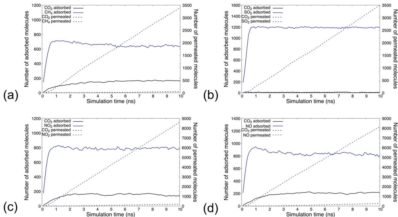
Fig. 4 Dynamic sorption and permeation profiles of gas mixtures comprised of 5 mol% CO<sub>2</sub> and (a) 95 mol% CH<sub>4</sub>, (b) 95 mol% SO<sub>2</sub>, (c) 95 mol% NO<sub>2</sub>, and (d) 95 mol% NO with respect to a rigid 4 × 4 × 3 MIL-160 membrane at 50 bar.
