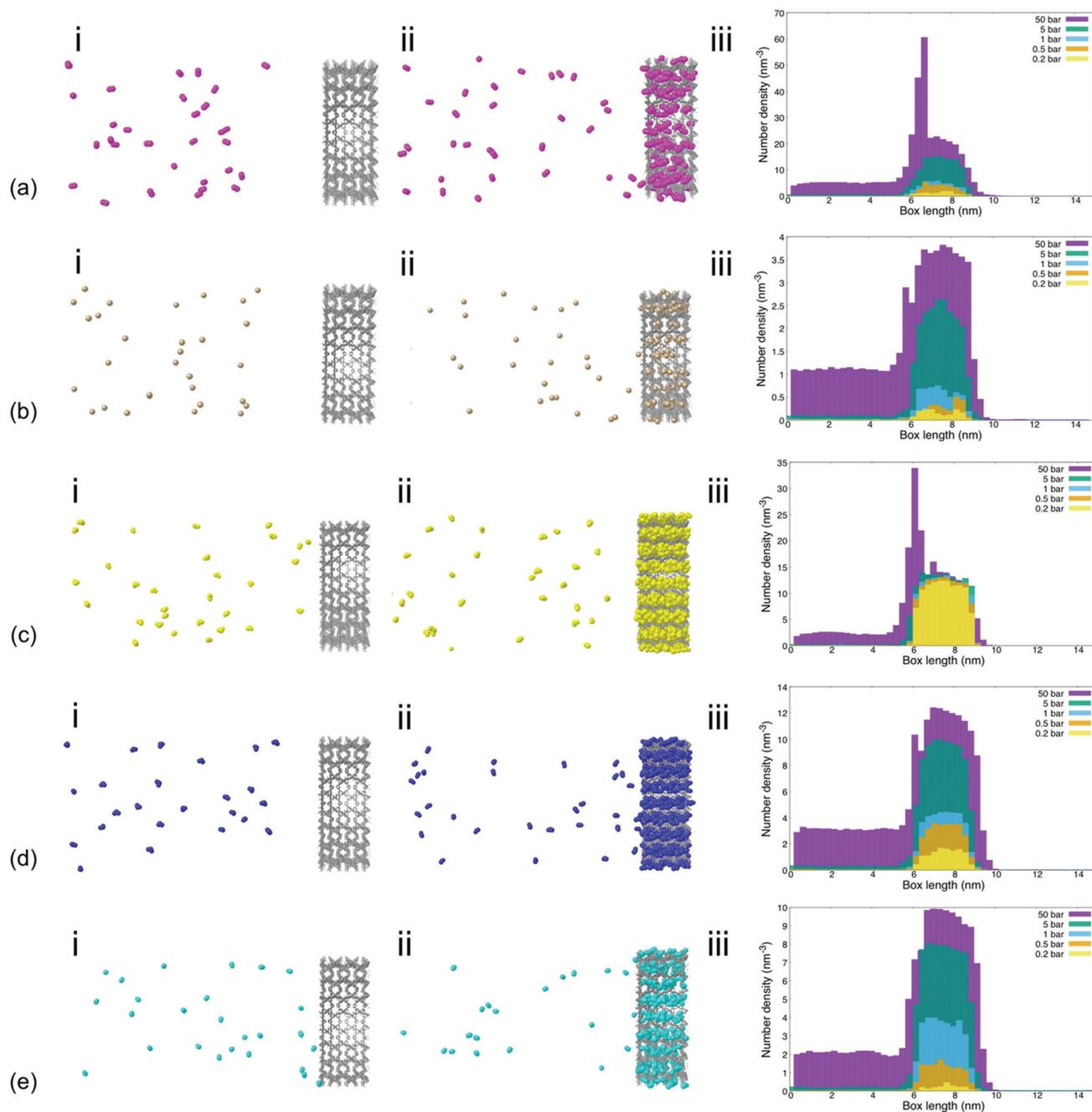
Fig. 2 (i) Initial configuration at 1 bar, (ii) steady-state configuration at 1 bar, and (iii) number density of gas species at steady state relative to the lateral direction of the simulation box at varied simulation pressures for (a) CO<sub>2</sub>, (b) CH<sub>4</sub>, (c) SO<sub>2</sub>, (d) NO<sub>2</sub>, and (e) NO.
