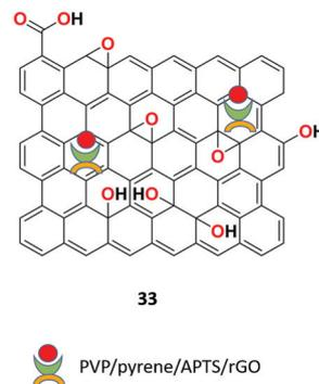
Fig. 36 The structure of PVP/pyrene/APTS/rGO fluorescent receptor **33**.
