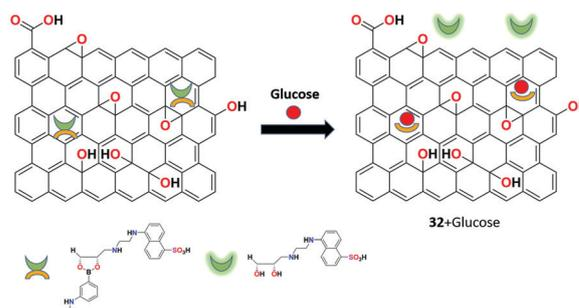
Fig. 35 Fluorescent detection of glucose molecule using receptor **32**.
