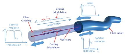
Fig. 13 FBG showing the sections where the core RI was increased, and typical reflection and transmission spectra
