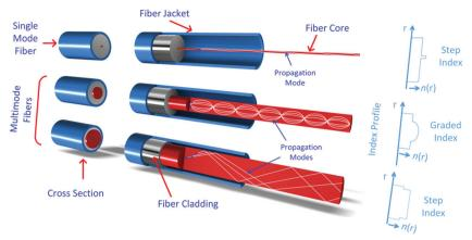
Fig. 11 Optical fiber types (i.e., multimode fiber and single mode fiber (SMF)).
