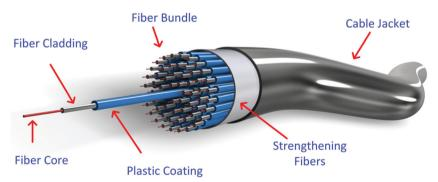
Fig. 10 Optical fiber in a bundle cable
