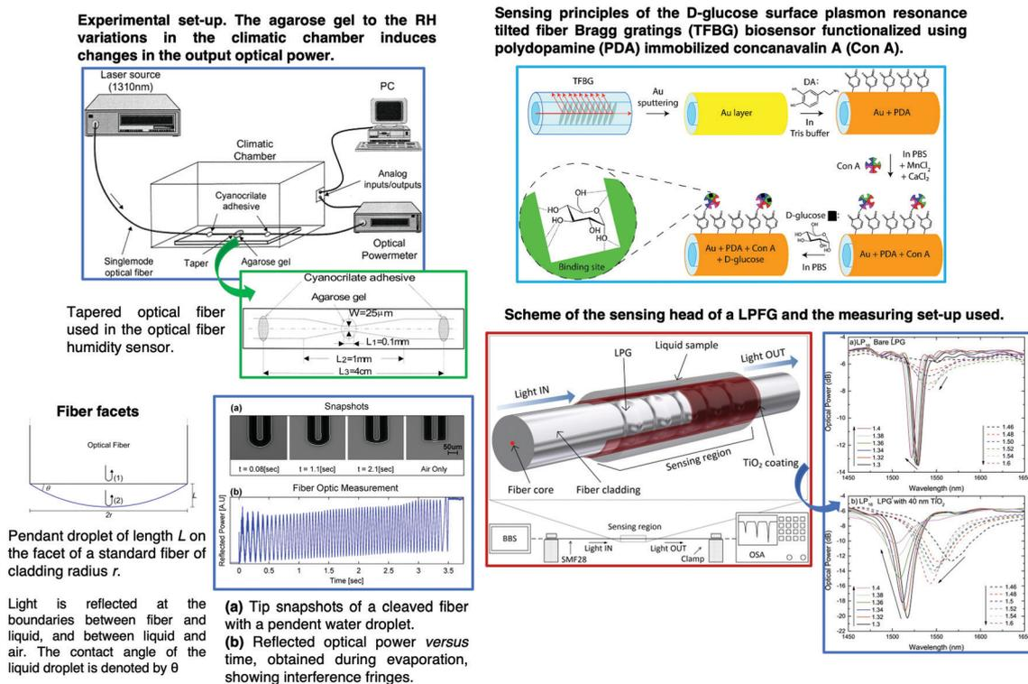
Fig. 15 Schematic of different OFS based on micro-structured optical fibers<sup>210</sup> or standard fibers with structural modifications, such as fiber tapers,<sup>211</sup> tilted FBGs, fiber facets<sup>215</sup> and LPFGs.<sup>216</sup> Reprinted and adapted with permission from ref. 211, 213–216. Copyright 2000 Elsevier. Copyright 2014 Elsevier. Copyright 2019 Elsevier.
