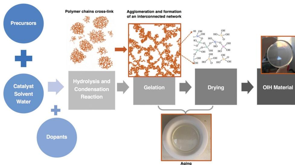
Fig. 6 Schematic of the main stages involved in the sol-gel method. Adapted from ref. 21.
