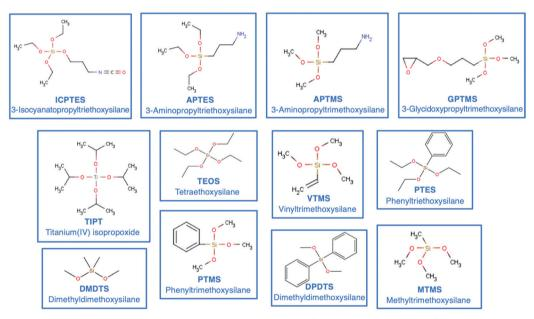
Scheme 1 Chemical structures and acronyms of the most common silicon alkoxides (including organic alkoxides) used as precursors in the synthesis of OIH materials.
