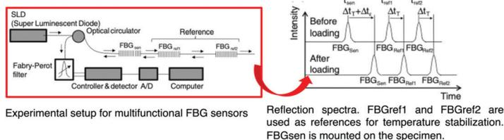
Experimental setup for multifunctional FBG sensors
