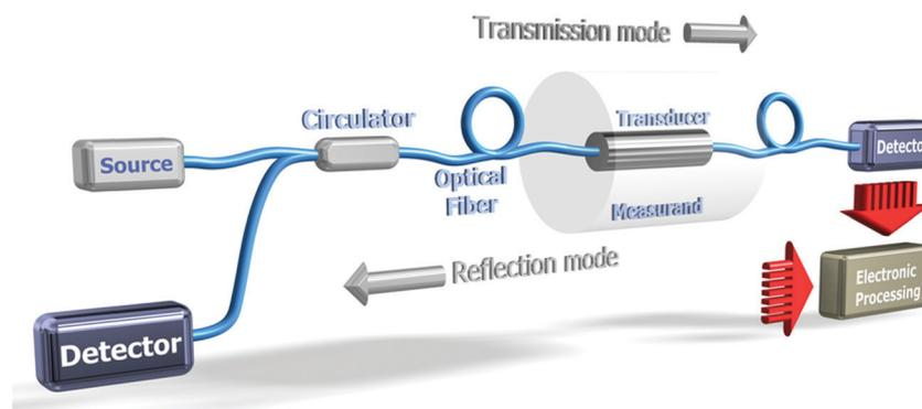
Fig. 12 Elementary building blocks of an OFS system.
