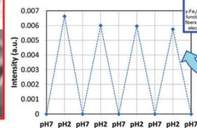
Reversibility of the pH-dependent on-off-on fluorescence intensity profile of electrospun magnetic fibers. The RT of the pH sensor was 30 s.
