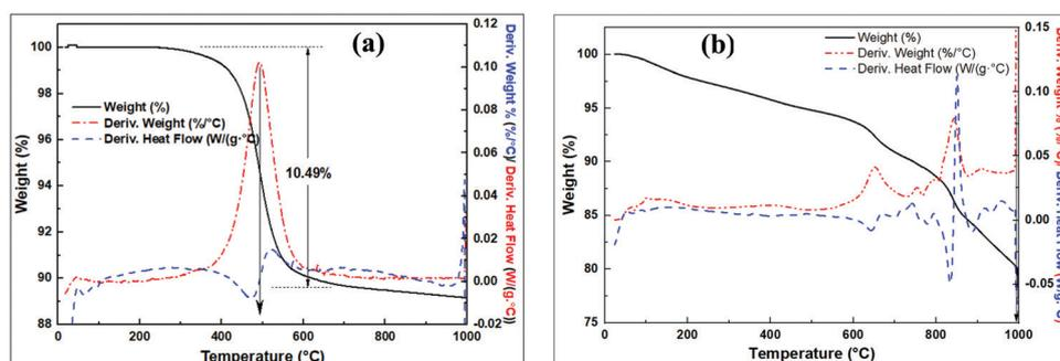
Fig. 3 TGA analysis of; (a) raw clay, (b) wet mixed raw clay with NaOH then dried.
