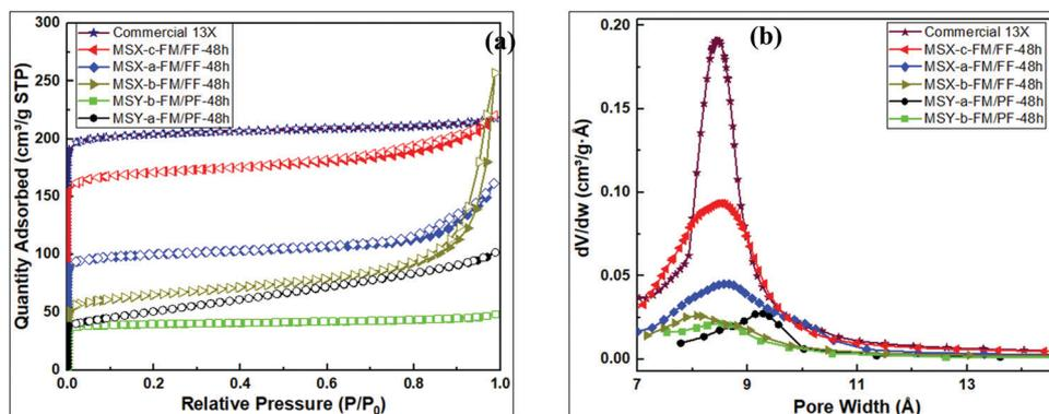
Fig. 8 Porosity analysis of synthesized zeolites; (a) N<sub>2</sub> sorption isotherms, (b) Horvath-Kawazoe pore size distribution curves.
