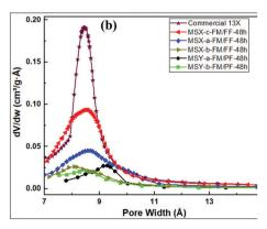
Fig. 8 Porosity analysis of synthesized zeolites; (a)  $N_2$  sorption isotherms, (b) Horvath–Kawazoe pore size distribution curves.
