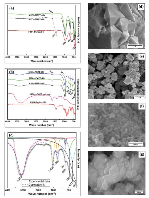
Fig. 4 The FTIR spectra of; (a) partial fusion products, (b) full fusion products, (c) deconvoluted FTIR peaks of the aged FF hydrogel modified with  $Na_2SiO_3-5H_2O$ , and SEM images of; (d) MSY-b-FM/PF-48h, (e) MSX-a-FM/FF-48h, (f) MSX-b-FM/FF-48h, (g) MSX-c-FM/FF-48h.
