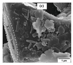
Fig. 2 Analysis of raw and pre-treated clay material; (a) FTIR spectra of raw clay, modified and F-MK, (b) XRD patterns of raw clay, modified and F-MK, (c) SEM image of raw clay
