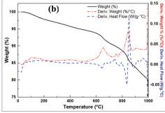
Fig. 3 TGA analysis of; (a) raw clay, (b) wet mixed raw clay with NaOH then dried.
