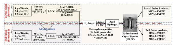
Fig. 1 Schematic for partial and full fusion protocols used for the synthesis of zeolites.
