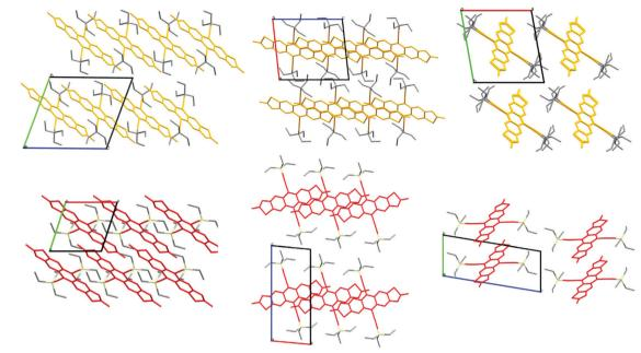
Crystal packing of TEC-FADT (orange, 1D, interdigitated side chains) and TES-FADT (red, 2D, interstack boundaries)
