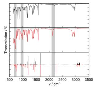
Fig. 3 Experimental FTIR spectra of TEC-FADT (top) and TES-FADT (middle), and computed vibrational frequencies and intensities (bottom, TEC-FADT in black and TES-FADT in red) using tuned  $\omega B97XD/6-31G^{\star}.$  Computed intensities for TEC-and TES-FADT are depicted with opposite sign for clarity.
