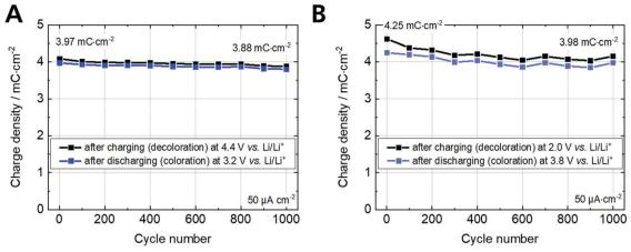
Fig. 5 Galvanostatic charging/discharging measurements with a current density of 50  $\mu$ A cm $^{-2}$  over 1000 switching cycles of (A) Fe-MEPE and (B) PB thin film electrodes on ultra-thin glass with Li as counter and reference electrode in 1 M LiClO<sub>4</sub>/PC as electrolyte.
