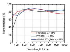
Fig. 1 Comparison of transmittance spectra of commercially available FTO glass (thickness: 4 mm) and PET-ITO films (127  $\mu$ m), and ultra-thin ITO glass (100 µm).
