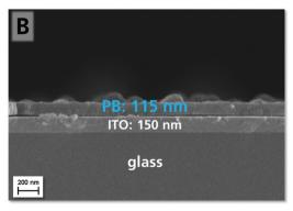
Fig. 2 SEM cross-section images depicting the thickness and interfaces of the (A) Fe-MEPE and (B) PB layer on ultra-thin ITO glass.
