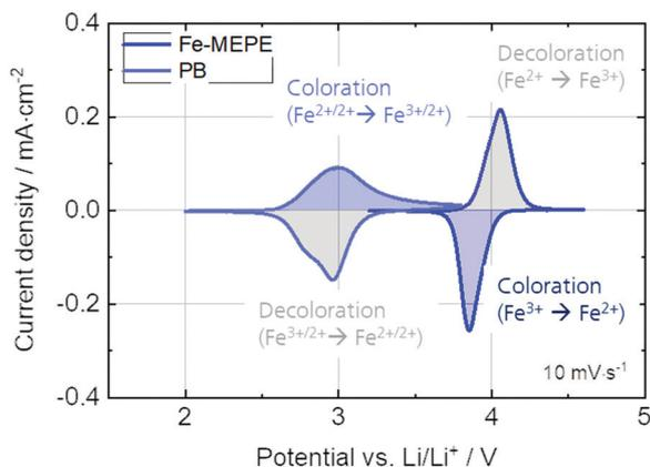
Fig. 4 Cyclic voltammograms (at 10 mV s<sup>-1</sup>) of the Fe-MEPE and PB thin film electrodes with Li as counter and reference electrode in 1 M LiClO<sub>4</sub>/PC as electrolyte.
