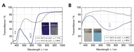
Fig. 3 Spectroelectrochemical characterization of (A) Fe-MEPE and (B) PB thin film electrodes with Li as counter and reference electrode in 1 M LiClO<sub>4</sub>/ PC as electrolyte
