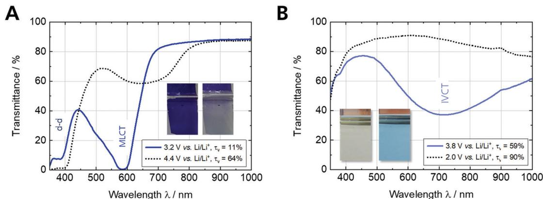
Fig. 3 Spectroelectrochemical characterization of (A) Fe-MEPE and (B) PB thin film electrodes with Li as counter and reference electrode in 1 M LiClO<sub>4</sub>/PC as electrolyte.
