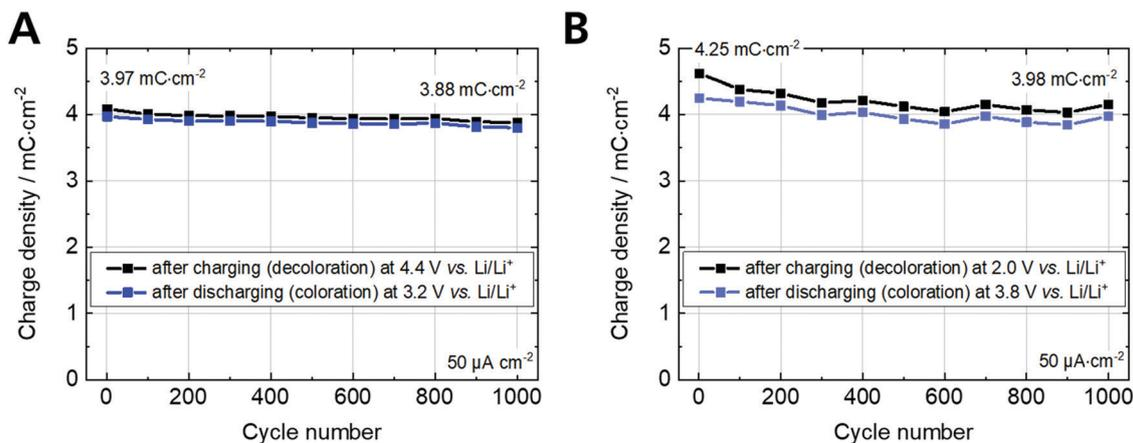
Fig. 5 Galvanostatic charging/discharging measurements with a current density of  $50 \mu\text{A cm}^{-2}$  over 1000 switching cycles of (A) Fe-MEPE and (B) PB thin film electrodes on ultra-thin glass with Li as counter and reference electrode in  $1 \text{ M LiClO}_4/\text{PC}$  as electrolyte.
