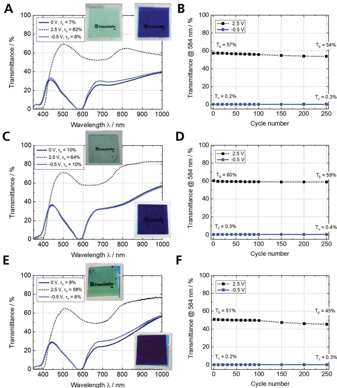
Fig. 6 Spectroelectrochemical characterization and change in transmittance at 584 nm over 250 potentiostatic cycles of the Fe-MEPE/PB ECDs (active area:  $3.5 \times 3.5 \text{ cm}^2$ ) on (A and B) FTO glass, (C and D) PET-ITO, and (E and F) ultra-thin ITO glass.
