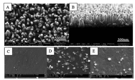
Fig. 12 (A and B) SEM images showing the surface morphology of rutile  $TiO_2$  nanorod arrays (TNA).<sup>139</sup> (C) SEM images showing the surface morphology of the ZrN film. (D and E) SEM images showing platelet adhesion on nickel-titanium SMA and ZrN film surfaces, respectively.<sup>141</sup> Adapted with permission from ref. 141. Copyright 2010, Elsevier.
