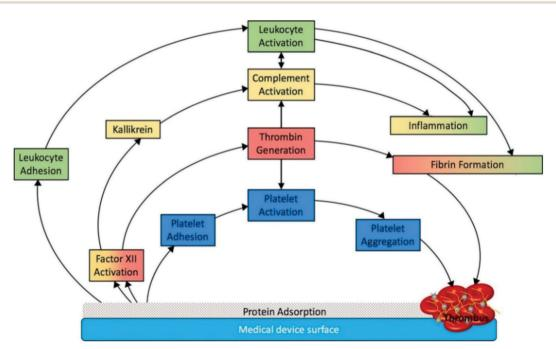
Fig. 3 Schematic representation of medical device associated thrombosis. 5 The initial protein adsorption on the implant surface mediates all the subsequent phenomena. Reproduced with permission from ref. 5. Copyright 2019, Elsevier.
