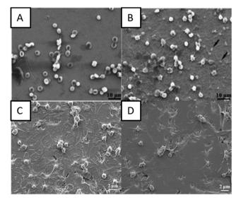
**Fig. 6** (A and B) SEM images of red blood cells on control surfaces and plasma oxidized surfaces at 280 W for 30 min, respectively. <sup>82</sup> SEM images showing the interaction of platelets with (C) titanium surfaces and (D) oxygen PIII treated surfaces. <sup>86</sup> Reproduced with permission from ref. 86. Copyright 2016, Elsevier.
