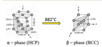
Fig. 2 Crystal structure transformation of titanium.<sup>28</sup> Adapted with permission from ref. 28. Copyright 2013, Elsevier.
