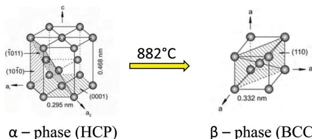
Fig. 2 Crystal structure transformation of titanium.<sup>28</sup> Adapted with permission from ref. 28. Copyright 2013, Elsevier.
