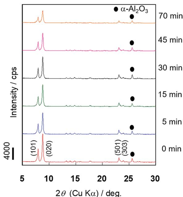
Fig. 4 XRD patterns of silicalite-1 membranes with different accumulated treatment periods.
