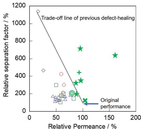
**Fig. 5** Relative separation factor as a function of relative permeance in various treated membranes: ○, TEOS;<sup>7,9</sup> △, TEFS;<sup>8</sup> ◇, TIPB;<sup>10</sup> □, Dye;<sup>11</sup> ☆, AT with CTAB (this study) for silicalite-1; +, for Na-BEA membrane; ⊙, for Na-MOR membrane; ×, for Na-ZSM-5 membranes.
