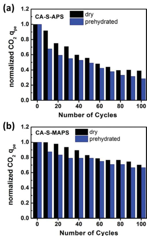
Fig. 24 Comparison of the cyclic CO<sub>2</sub> capacity of dry fibres and prehydrated fibres in 200 ppm SO<sub>2</sub> in 10% CO<sub>2</sub>/N<sub>2</sub> at 35 °C of; (a) primary amine-grafted and; (b) secondary amine-grafted fibres. CO<sub>2</sub> capacities normalised to adsorbents' initial CO<sub>2</sub> capacity  $q_{pe,0}$  before exposure degradation. Reprinted from ref. 36 Copyright (2015), with permission from Elsevier.
