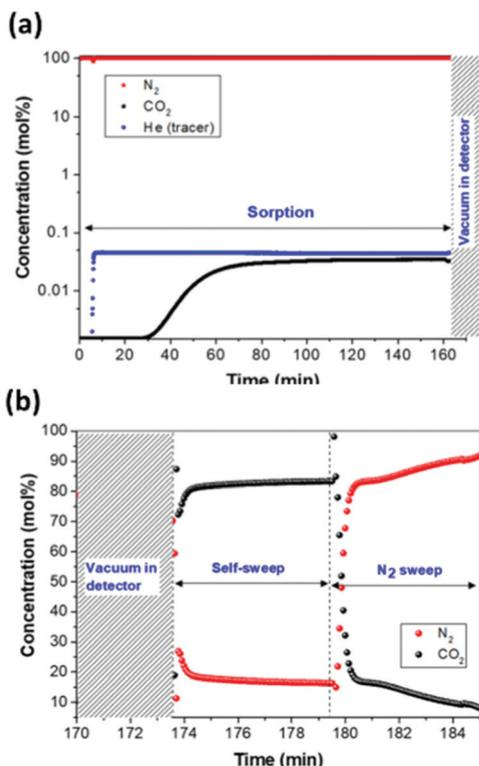
Fig. 25 (a) Breakthrough profile of PEI-functionalised cellulose acetate/silica fibres during CO<sub>2</sub> adsorption under dry 380 ppm CO<sub>2</sub>/395 ppm He/balance N<sub>2</sub> at 35 °C. (b) Concentration profiles during the 'self-sweep' and N<sub>2</sub> sweep stages of desorption. Reprinted with permission from ref. 39. Copyright (2019) American Chemical Society.
