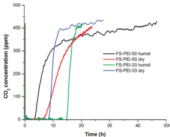
Fig. 9 Adsorption of CO<sub>2</sub> from the air at 25 °C on FS-PEI-50 and FS-PEI-33 under dry and humid conditions, illustrating longer period before breakthrough for FS-PEI-33 (33 wt% polyamine loading). Reprinted with permission from ref. 32 Copyright (2011) American Chemical Society.
