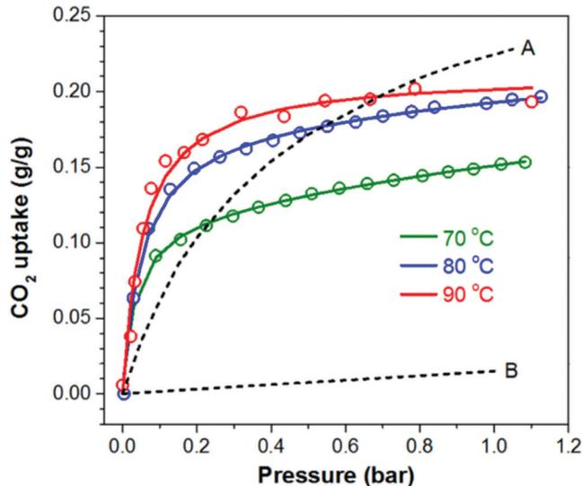
Fig. 15 CO<sub>2</sub> uptake isotherms of PEI–C60 at 70 °C, 80 °C and 90 °C and compared to the absorption of CO<sub>2</sub> on (A) Mg-MOF-74 and (B) MOF-177, both at 90 °C. Reproduced from ref. 106 according to Creative Commons Attribution 4.0 International (CC BY 4.0).
