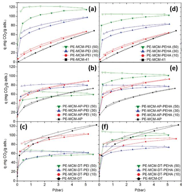
Fig. 13 Pure CO<sub>2</sub> adsorption–desorption isotherms at 45 °C of pore-expanded-MCM-41 support impregnated with (a) PEI and (b) modified by double functionalisation with AP, or (c) DT. Or impregnated with (d) PEHA and (e) modified by double functionalisation with AP, or (c) DT. Adapted from ref. 128, copyright (2014), with permission from Elsevier.
