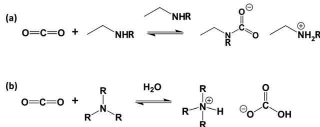
Fig. 2 Mechanism of reaction of CO<sub>2</sub> with (a) primary- or secondary- amines in the absence of water and (b) tertiary amines in the presence of water.
