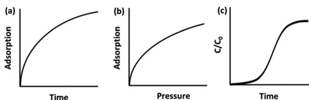
Fig. 1 Typical graphs of raw data obtained for CO<sub>2</sub> adsorption *via* (a) gravimetric; (b) volumetric; and (c) breakthrough analyses.
