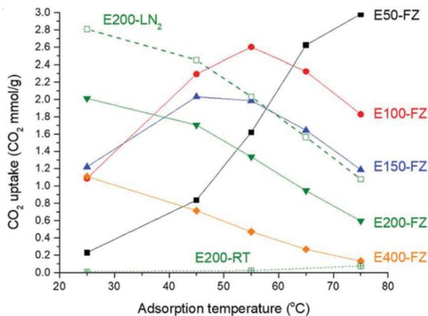
Fig. 11 Variation in CO<sub>2</sub> capacity with temperature for different amine/cross-linker compositions. Adsorption under 10% CO<sub>2</sub> for 3 hours. Reproduced from ref. 117 with permission from the Royal Society of Chemistry.
