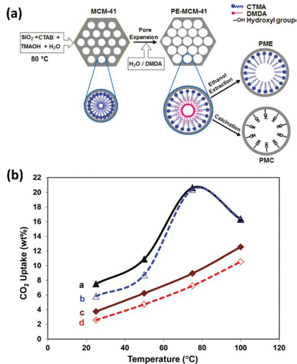
Fig. 12 (a) Schematic representation of the syntheses of PME and PMC. (b) CO<sub>2</sub> uptake versus temperature for (a) PME-PEI(55) after 180 min, (b) PME-PEI(55) after 30 min, (c) PMC-PEI(55) after 180 min, and (d) PMC-PEI(55) after 30 min of exposure to pure CO<sub>2</sub>. Adapted with permission from ref. 127. Copyright (2011) American Chemical Society.
