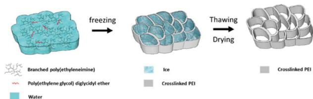
Fig. 8 Schematic synthesis of self-supported adsorbent synthesised from cross-linking PEI ( $M_w$  750 000 Da) with poly(ethylene glycol). Reproduced from ref. 117 with permission from the Royal Society of Chemistry.
