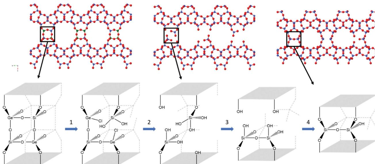
Fig. 7 The four steps observed in the hydrolysis of UTL with 6 M hydrochloric acid, with the crystallographic representation (top) and the d4r highlighting key bond breakages and formation (bottom). In the crystal structure, blue represents silicon, green for germanium and red for oxygen. The four key steps show the attack of chloride at the germanium d4r atoms (1), removal of germanium (2), silicon rearrangement (3) and condensation of silanol groups (4).
