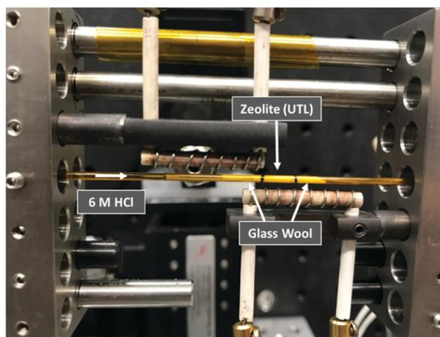
**Fig. 2** The experimental set-up of the *in situ* flow hydrolysis of zeolite **UTL**. The zeolite was held in place between two plugs of glass wool, with the sample region denoted by the black lines, and the acid pumped through the sample.
