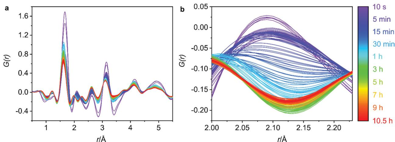
Fig. 3 (a) The 0.5–5.5 Å region of the 6 M hydrochloric acid hydrolysis of **UTL**. (b) The Ge–Cl interatomic distance that decreases over time as germanium is removed from the **UTL** framework. The Ge–Cl product is removed due to the flow nature of the experiment.
