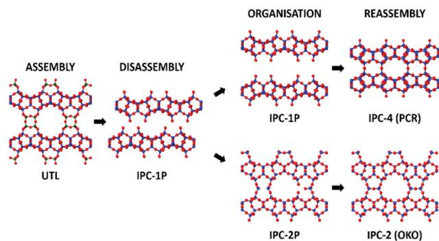
**Fig. 1** An overview of two different routes in the ADOR process showing the assembly, disassembly, organisation, and reassembly of the parent zeolite **UTL** to final products **IPC-4** and **IPC-2**. Blue atoms represent the T-atoms within the layers, which are predominantly silicon, dark green represents T-atoms of the double 4 rings (d4r) that are a combination of silicon and germanium, where the ratio is dependent upon synthesis conditions, and red are oxygen atoms.
