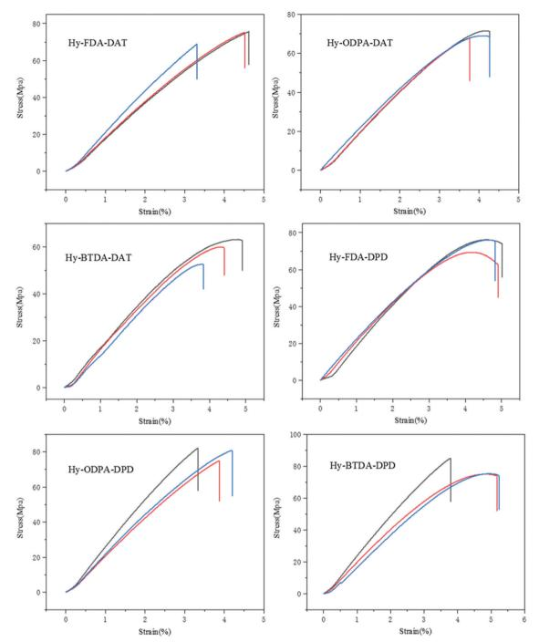
Fig. 1 Tensile stress-strain curves of the as-synthesized hybrid films. Three different samples were tested for each material.
