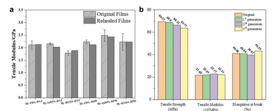
Fig. 3 (a) Tensile moduli of six hybrid films before and after repairing; (b) mechanical properties of Hy-ODPA-DAT after three generation recycling.
