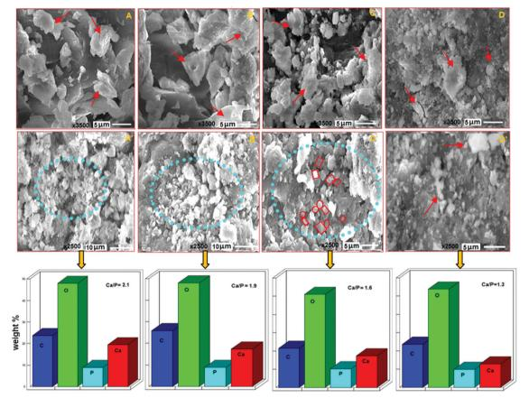
Fig. 3 Characteristic SEM micrographs illustrating the bioactivity profile by the SBF study of [A] BCHD1, [B] BCHD2, [C] BCHD3, and [D] CH nanocomposite scaffolds at 4 weeks [magnification: ×3500, scale bar: 5 μm] and at 8 weeks [A'-D'] [magnification: ×2500, scale bar: 10 μm], respectively, with their respective EDX micrographs recorded after 8 weeks
