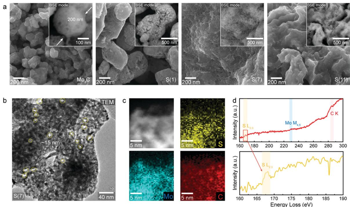
**Fig. 2** Characterization observations of as-synthesized sulfur doped molybdenum carbides. (a) Morphology investigation with scanning electron microscopy (SEM) depending on sulfur doping concentrations: Mo<sub>2</sub>C, S(1), S(7) and S(11). (b) Transmission electron microscopy (TEM) image of S(7) to demonstrate porous morphology and pore size. (c) Electron energy loss spectroscopy (EELS) mapping image of S(7) and (d) element spectrum of fabricated sulfur doped Mo<sub>2</sub>C.
