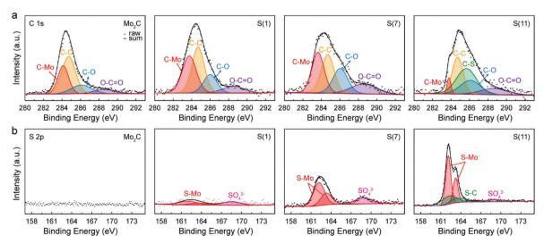
Fig. 4 X-Ray photoelectron spectroscopy (XPS) observations with fabricated catalysts. (a) C 1s spectra and (b) S 2p spectra of Mo<sub>2</sub>C, S(1), S(7), and S(11).
