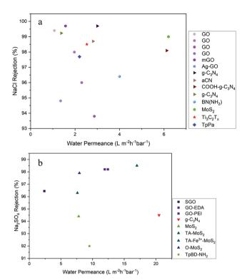
Fig. 3 Performance of 2D-enabled TFN membranes for (a) NaCl rejection and (b) Na<sub>2</sub>SO<sub>4</sub> rejection.
