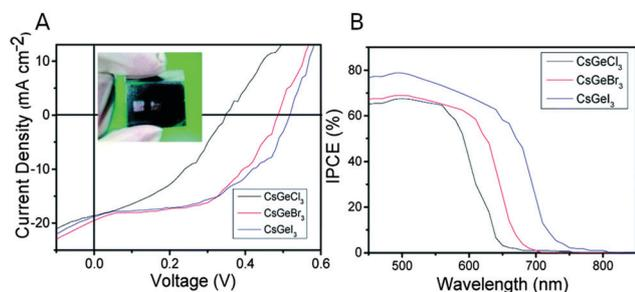
Fig. 4 (A)  $J$ – $V$  characteristics of  $\text{CsGeI}_3$  (blue),  $\text{CsGeBr}_3$  (red), and  $\text{CsGeCl}_3$  (black) solar cells. The inset shows a picture of a solar cell. (B) Incident Photon-to-electron Conversion Efficiency (IPCE) of  $\text{CsGeX}_3$  perovskite devices with different halides. Reproduced from ref. 80 with permission from the Royal Society of Chemistry. (RSC, RSC Advances).
