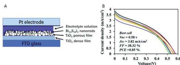
Fig. 5 (A) Scheme of the Bi<sub>13</sub>S<sub>18</sub>I<sub>2</sub> NCs solar cell structure. (B) *J*-*V* curves of eight Bi<sub>13</sub>S<sub>18</sub>I<sub>2</sub> solar cells. Reproduced from ref. 100 with permission from the Royal Society of Chemistry. (RSC, Journal of Materials Chemistry C).
