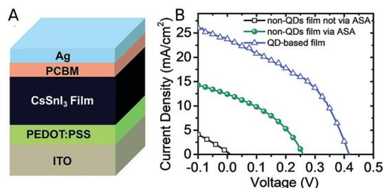
Fig. 3 (A) Device structure of the solar cell based on the  $\text{CsSnI}_3$  films. (B)  $J$ - $V$  curves of  $\text{CsSnI}_3$  bulk solar cell (black),  $\text{CsSnI}_3$  bulk solar cell with the addition of TPPi as antioxidant additive (green) and  $\text{CsSnI}_3$  NCs solar cell with TPPi (blue). Reproduced from ref. 58 with permission from the Royal Society of Chemistry (RSC, Journal of Materials Chemistry A).
