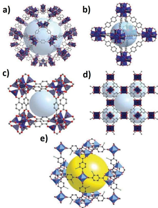
Fig. 9 Typical structure of representative MOFs: MIL-101 (a), UiO-67 (b) MOF-5 (c), HKUST-1 (d)<sup>125</sup> and MOF-101 (e).<sup>126,127</sup>
