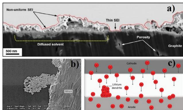
Fig. 5 Scanning electron microscopy (SEM) image of the SEI layer in a LIB anode<sup>54</sup> (a) SEM image of a lithium dendrite<sup>55</sup> (b); schematic representation of the lithium dendrite formation process (c).
