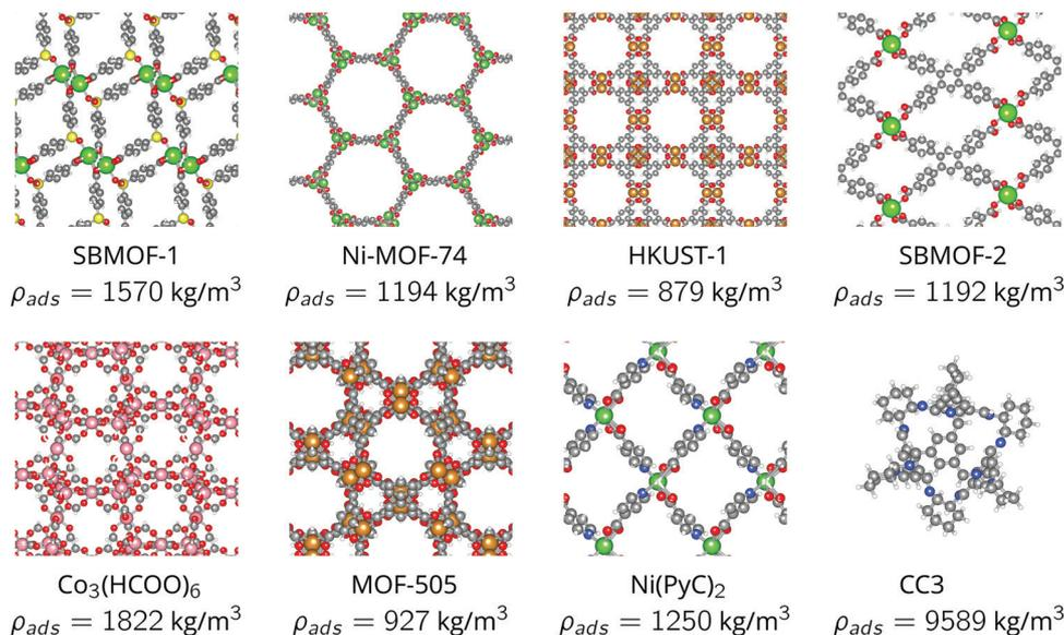
Fig. 4 The crystal structures of the nanoporous material candidates we consider for adsorbed xenon propellant storage and their (crystal) densities,  $\rho_{ads}$ . For CC3, a molecular material, we show only a single cage.
