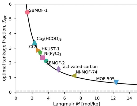
Fig. 7 The relationship between the tankage fraction of each optimized adsorbed xenon storage system and the saturation loading of xenon in the adsorbent,  $M$ . The solid curve shows the approximation to the optimal tankage fraction in eqn (13).
