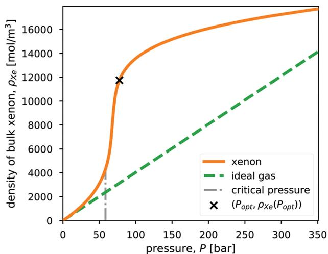
**Fig. 2** The density of xenon,  $\rho_{\text{Xe}} = \rho_{\text{Xe}}(P)$ , as a function of pressure,  $P$ , at a fixed temperature of 298 K, taken from NIST.<sup>26</sup> For comparison, the density of the ideal gas is also shown. The vertical, dashed line marks the critical pressure of xenon ( $P_c = 58.42$  bar. Note  $T_c = 289.74$  K.). The x marks the optimal storage conditions in a bulk xenon propellant storage system, which we will derive later.
