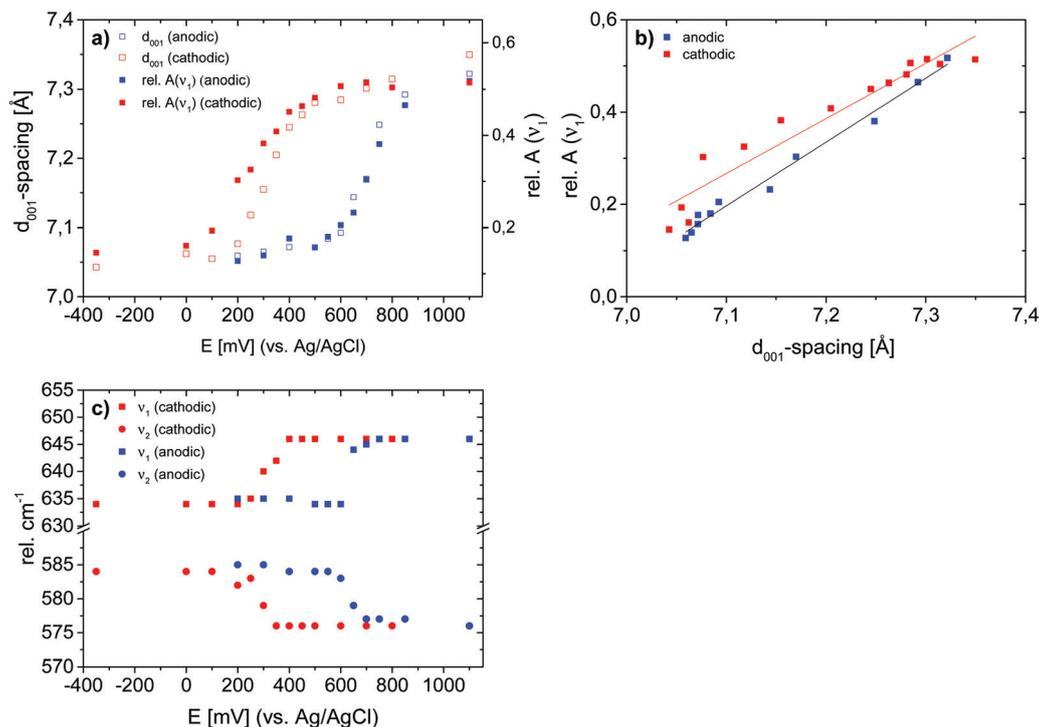
Fig. 10 (a) Potential dependent evolution of the  $d_{001}$ -spacing and rel.  $A(\nu_1)$ . (b) Potential dependent evolution of rel.  $A(\nu_1)$  as a function of the interlayer spacing ( $d_{001}$ -spacing). (c) Potential dependent evolution of the position of the Raman bands  $\nu_1$  and  $\nu_2$ . Electrolyte was 0.5 M  $\text{Na}_2\text{SO}_4$ .
