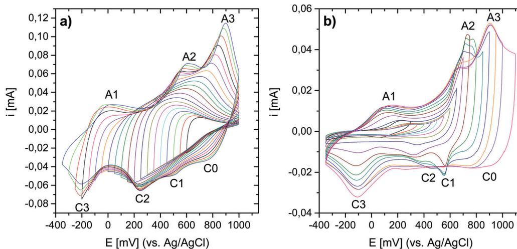
Fig. 6 (a) CV curves measured at  $10 \text{ mV s}^{-1}$  starting from  $1000 \text{ mV}$  and with a continuously widened potential window down to  $-350 \text{ mV}$ . (b) CV curves measured starting from  $-350 \text{ mV}$  and with a continuously widened potential window up to  $1100 \text{ mV}$ . Electrolyte:  $0.5 \text{ M Na}_2\text{SO}_4$ . Scan rate:  $10 \text{ mV s}^{-1}$ .
