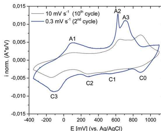
**Fig. 5** Normalized cyclic voltammograms of Li,Na,K-bir in 0.5 M  $\text{Na}_2\text{SO}_4$  aqueous electrolyte (potential window:  $-350 \text{ mV}$ – $1100 \text{ mV}$  vs. Ag/AgCl) measured at different scan rates:  $10 \text{ mV s}^{-1}$  (black) and  $0.3 \text{ mV s}^{-1}$  (blue).
