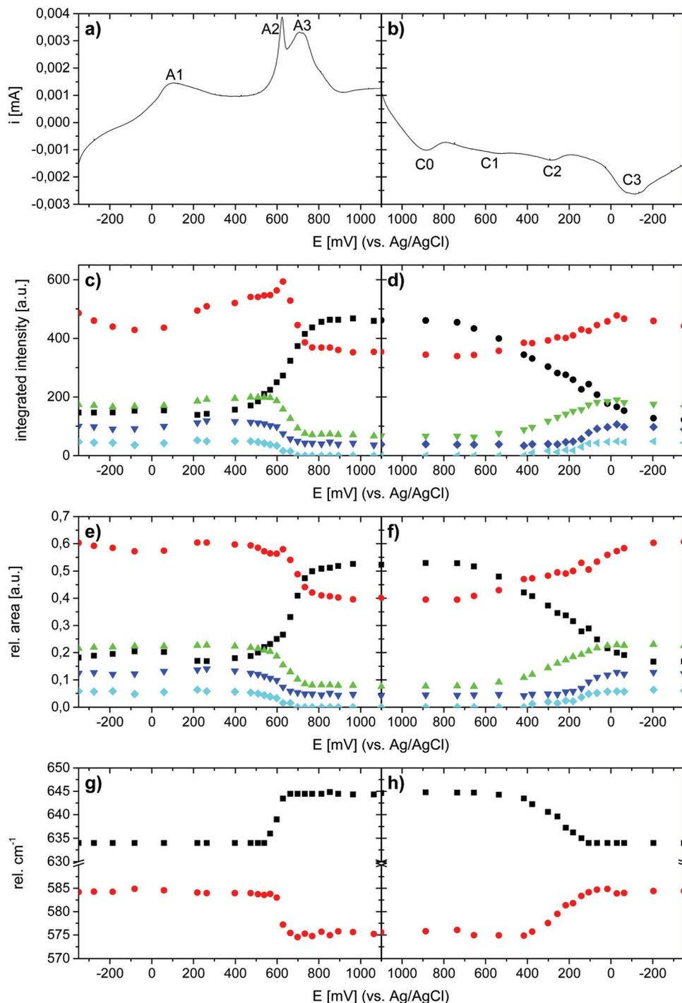
**Fig. 9** Potential dependent evolution of the individual Raman bands in the course of a CV cycle in 0.5 M Na<sub>2</sub>SO<sub>4</sub>, obtained from deconvolution. (a) and (b) CV-curves. (c) and (d) Integrated intensities. (e) and (f) Rel. integrated intensities. (g) and (h) Spectral positions of  $\nu_1$  and  $\nu_2$ . Scan rate: 0.3 mV s<sup>-1</sup>.  $\nu_1$  (■),  $\nu_2$  (●),  $\nu_3$  (▲),  $\nu_4$  (▼), and  $\nu_5$  (◆).
