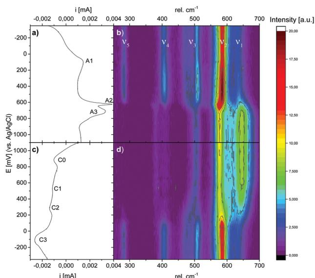
Fig. 7 (a) Anodic and (c) cathodic potential scans. Scan rate: 0.3 mV s<sup>-1</sup>, electrolyte: 0.5 M Na<sub>2</sub>SO<sub>4</sub>. (b) and (d) contour plots showing simultaneous changes in the Raman spectral peak intensities for electrochemically activated birnessite MnO<sub>2</sub>.
