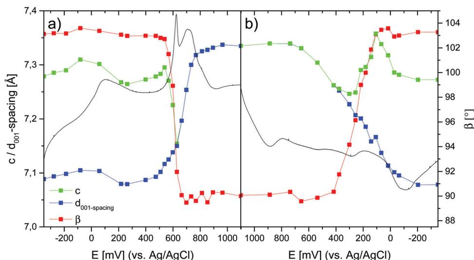
Fig. 11 Potential dependent evolution of  $\beta$  (red) and  $d_{001}$ -spacing (blue), calculated based on the positions of the  $\nu_1$  and  $\nu_2$  bands ( $\Delta(\nu_1 - \nu_2)$ ) and the relative integrated intensity of  $\nu_1$ , respectively. The lattice parameter  $c$  (green) was calculated based on  $\beta$  and the  $d_{001}$ -spacing. The current trace is included in arbitrary units for clarity.
