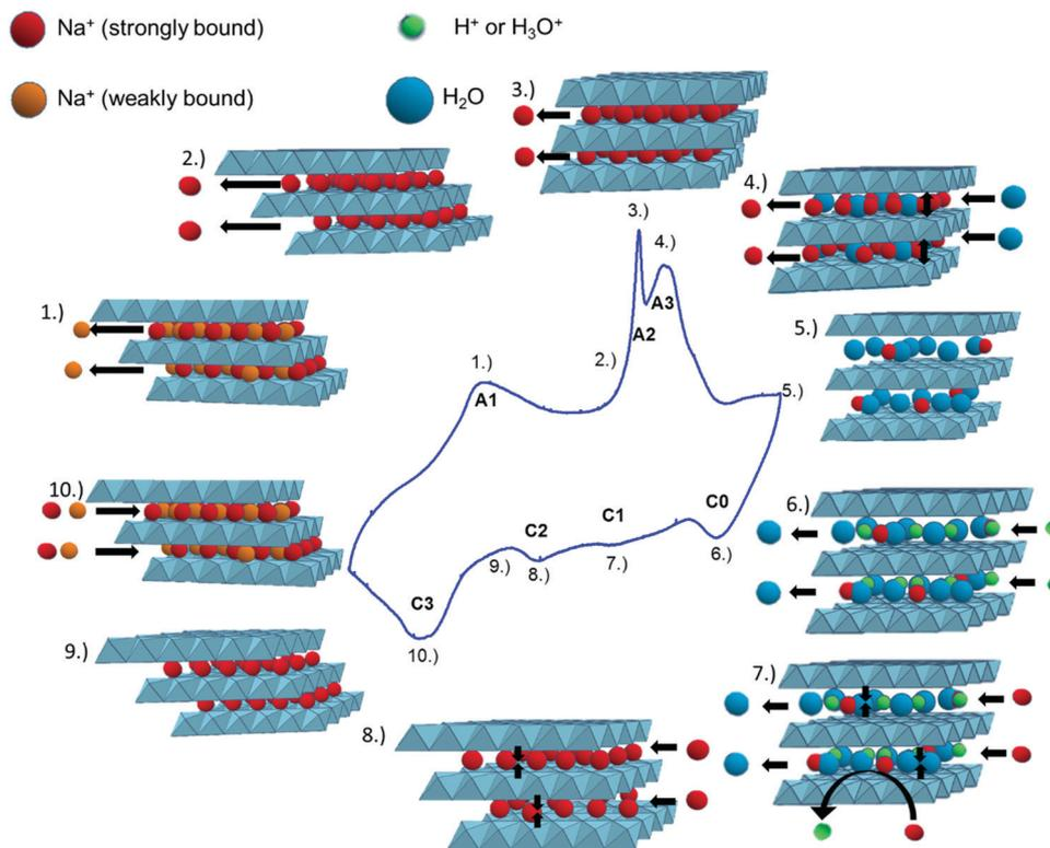
Fig. 12 Proposed mechanism of Na<sup>+</sup> deintercalation (anodic scan), and intercalation (cathodic scan) in birnessite, and its connection to the CV curve. See the text for details.
