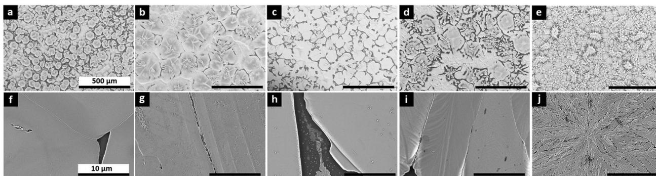
**Fig. 2** SEM images of  $\text{MAPb}_{0.5}\text{Sn}_{0.5}\text{I}_3$  with 0% (a; f), 0.1% (b; g), 0.2% (c; h), 1% (d; i) and 5% (e; j) F4TCNQ dopant, using an Everhart–Thornley detector with  $100\times$  magnification (a to e) and a Trinity detector with  $5000\times$  magnification collecting mostly secondary electrons (f to j). The scale bar is  $500\ \mu\text{m}$  for (a) to (e) and  $10\ \mu\text{m}$  for (f) to (j).
