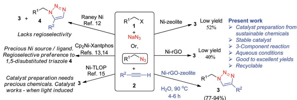
Scheme 1 Comparative scheme for various Ni-catalysed azide alkyne cycloadditions either in two- or three-component processes.
