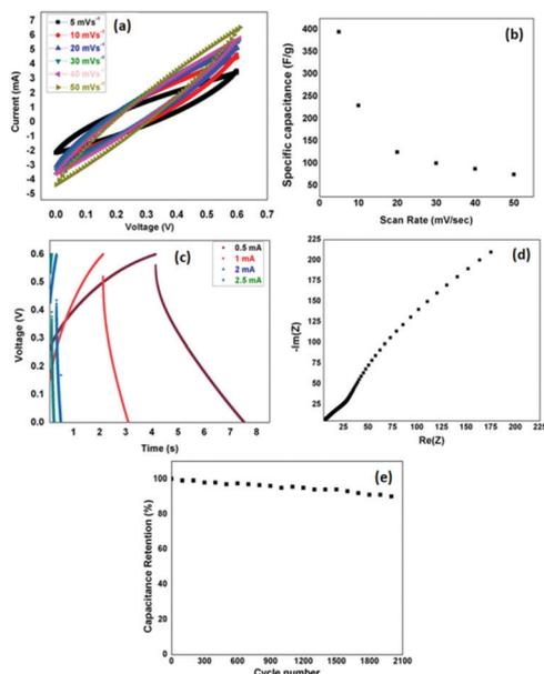
Fig. 4 (a) CV curves recorded at the scan rate of 5, 10, 20, 30, 40, and 50  $\text{mV s}^{-1}$ , (b) Specific capacitance as a function of scan rate, (c) Charging and discharging curves measured at current densities of 0.5, 1, 2 and 2.5 mA, (d) Nyquist plot, and (e) cycle stability of CC- $\text{Co}_3\text{O}_4$  respectively.
