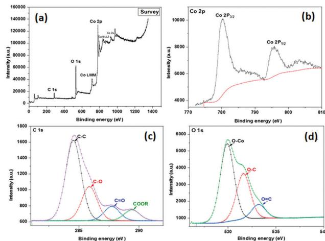
Fig. 3 XPS of CC-CO<sub>3</sub>O<sub>4</sub> (a) Survey scan, (b) Co 2p spectrum, (c) C 1s spectrum, and (d) O 1s spectrum.
