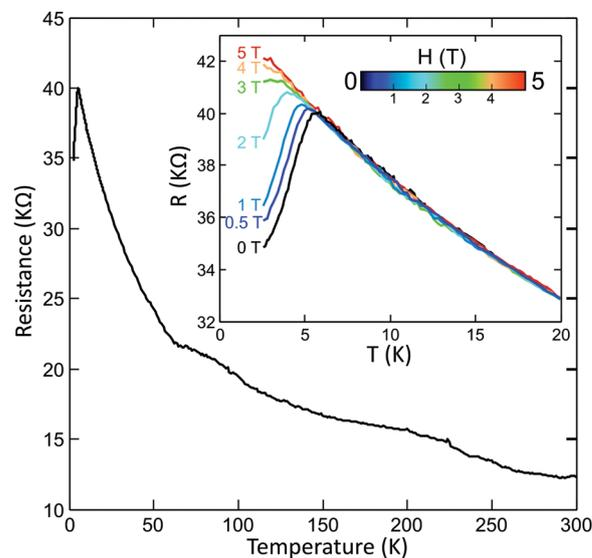
Fig. 3 Temperature dependent resistance of a NbSe<sub>2</sub> film on standard copy paper. (a) Resistance vs. temperature measured on a NbSe<sub>2</sub>-on-paper film at zero-field (sample 3, van der Pauw geometry). (Inset) Resistance vs. temperature curves measured at different applied magnetic fields.
