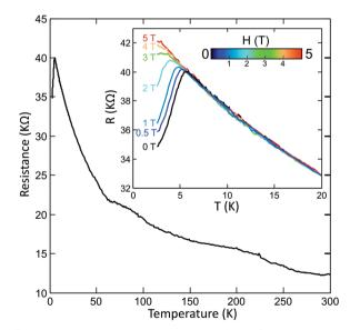
Fig. 3 Temperature dependent resistance of a NbSe<sub>2</sub> film on standard copy paper. (a) Resistance vs. temperature measured on a NbSe2-onpaper film at zero-field (sample 3, van der Pauw geometry). (Inset) Resistance vs. temperature curves measured at different applied magnetic
