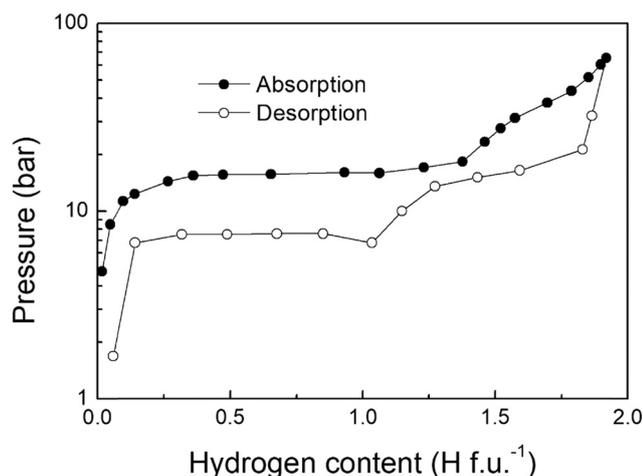
Fig. 4 Pressure-composition-isotherm of TiFe performed at 40 °C.
