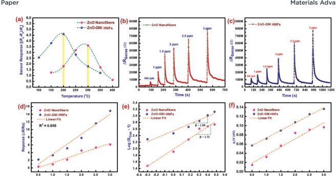
Fig. 6 (a) Sensor response graph of NO<sub>2</sub> versus different temperature, (b and c) NO<sub>2</sub> sensor response-recovery plots of pristine ZnO and aligned heterojunction ZnO-GNI HNFs at its operational temperature, (d) sensor response against NO<sub>2</sub> concentration, (e)  $\log(S_{\rm qas}-1)$  versus  $\log(P_{\rm qas})$  plot toward 0.5-3 ppm of NO<sub>2</sub> gas and (f) effect of band bending upon increasing NO<sub>2</sub> concentration
