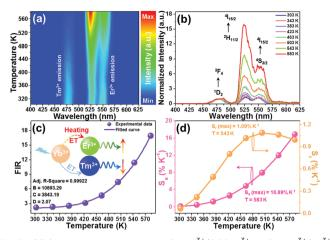
Fig. 5 (a) Contour lines of the  $Y_2Mo_3O_{12}$ :  $Er^{3+}/0.22Yb^{3+}$ @BiOF: $Tm^{3+}/Yb^{3+}$ (i.e., mass rate = 1:5) composites as a function of temperature excited at 980 nm. (b) Temperature-dependent UC emission spectra (normalized at 480 nm) and (c) FIR value of the  $Y_2Mo_3O_{12}$ :  $Er^{3+}/0.22Yb^{3+}$ @BiOF: $Tm^{3+}/0.22Yb^{3+}$  $Yb^{3+}$  composites. (d) Dependence of the  $S_a$  and  $S_r$  values on the temperature
