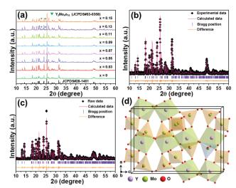
Fig. 1 (a) XRD patterns of the  $Y_2Mo_3O_{12}$ : $Er^{3+}/2xYb^{3+}$  microparticles. Rietveld XRD refinement patterns of the (b)  $Y_2Mo_3O_{12}$ : $Er^{3+}$  and (c)  $Y_2Mo_3O_{12}$ : $Er^{3+}/0.22Yb^{3+}$  microparticles. (d) Crystal structure of the  $Y_2Mo_3O_{12}$  unit cell.
