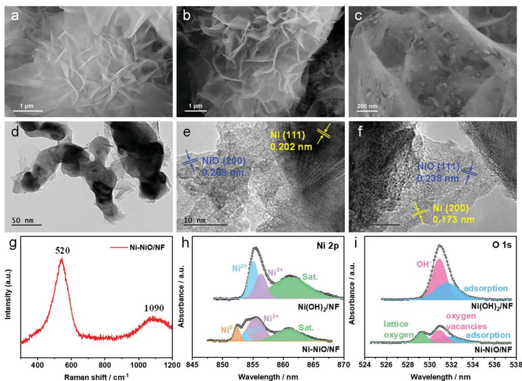
Fig. 1 (a) SEM image of the precursor  $\text{Ni}(\text{OH})_2/\text{NF}$ . (b) Low-magnification SEM image, (c) high-magnification SEM image, (d) TEM image, and (e and f) HRTEM image of Ni-NiO/NF. (g) Raman spectrum of Ni-NiO/NF. XPS spectra of (h) Ni 2p and (i) O 1s in the sample of Ni-NiO/NF.
