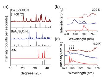
Fig. 5 PXRD patterns of Ca- $\alpha$ -SiAlON (1400 °C), BaAl $_3$ Si $_3$ O $_4$ N $_5$  and AlN (a), Mn $^{2+}$  PL in respective samples at 300 K (b) and at 4.2 K (c) under 275 nm excitation. In (a), the gray colored patterns represent reference diffraction patterns ( $\lambda_{K\alpha}=1.5401$  Å). The samples are identified using line colors as indexed in (a). In (c), the dotted arrows point position of vibronic side bands
