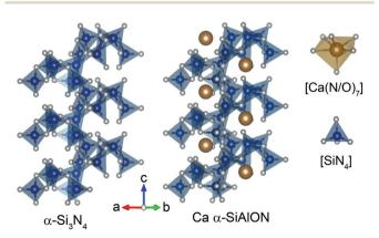
Fig. 1 Crystal structure of  $\alpha$ -Si<sub>3</sub>N<sub>4</sub> and Ca- $\alpha$ -SiAlON along c-axis. The brown, blue and gray spheres represent Ca, Si/Al, and N/O ions, respectively. The coordination polyhedron of Ca and Si tetrahedron are presented in right side.
