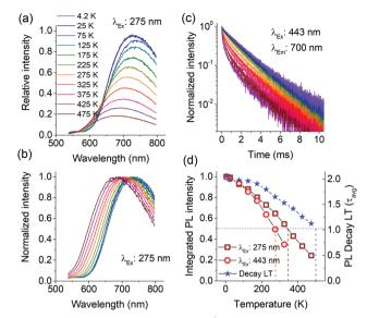
Fig. 4 Temperature dependent PL of  $Mn^{2+}$  (10 at%) doped  $Ca-\alpha$ -SiAlON under 275 nm excitation (a); PL in normalized scale (b); PL decay curves (c); and the plot of integrated PL intensity (under 275 nm and 443 nm excitations) and the PL decay time with temperature (d). In (a), (b) and (c), the line colors are as indexed in (a). In (d), the integrated PL values were derived from 535-800 nm spectral range.
