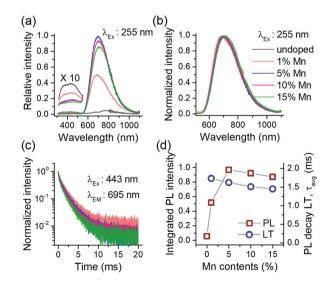
Fig. 3 Concentration dependent PL (a); PL spectra in normalized scale (b); PL decay curves (c); and the plot of integrated PL intensity and luminescence decay times vs. concentration in  $Mn^{2+}$  activated Ca- $\alpha$ -SiAlON (d). In (a), (b) and (c), the line colors as indexed in (b) identify respective concentrations.
