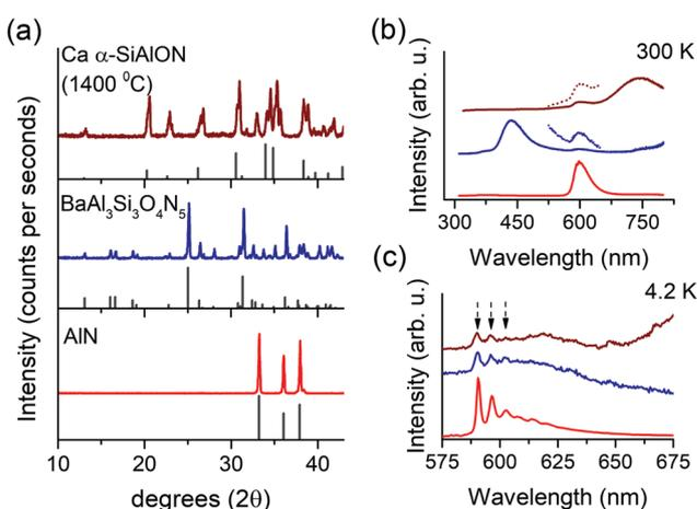
Fig. 5 XRD patterns of  $\text{Ca-}\alpha\text{-SiAlON}$  (1400 °C),  $\text{BaAl}_3\text{Si}_3\text{O}_4\text{N}_5$  and  $\text{AlN}$  (a),  $\text{Mn}^{2+}$  PL in respective samples at 300 K (b) and at 4.2 K (c) under 275 nm excitation. In (a), the gray colored patterns represent reference diffraction patterns ( $\lambda_{\text{K}\alpha} = 1.5401 \text{ \AA}$ ). The samples are identified using line colors as indexed in (a). In (c), the dotted arrows point position of vibronic side bands.
