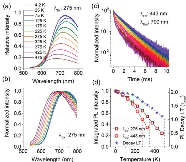
Fig. 4 Temperature dependent PL of  $\text{Mn}^{2+}$  (10 at%) doped  $\text{Ca-}\alpha\text{-SiAlON}$  under 275 nm excitation (a); PL in normalized scale (b); PL decay curves (c); and the plot of integrated PL intensity (under 275 nm and 443 nm excitations) and the PL decay time with temperature (d). In (a), (b) and (c), the line colors are as indexed in (a). In (d), the integrated PL values were derived from 535–800 nm spectral range.
