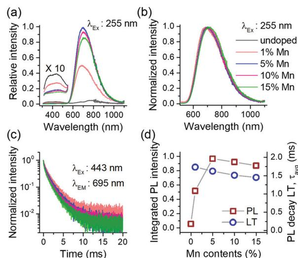
**Fig. 3** Concentration dependent PL (a); PL spectra in normalized scale (b); PL decay curves (c); and the plot of integrated PL intensity and luminescence decay times vs. concentration in Mn<sup>2+</sup> activated Ca- $\alpha$ -SiAlON (d). In (a), (b) and (c), the line colors as indexed in (b) identify respective concentrations.
