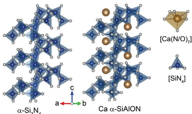
Fig. 1 Crystal structure of  $\alpha$ - $\text{Si}_3\text{N}_4$  and Ca- $\alpha$ -SiAlON along *c*-axis. The brown, blue and gray spheres represent Ca, Si/Al, and N/O ions, respectively. The coordination polyhedron of Ca and Si tetrahedron are presented in right side.
