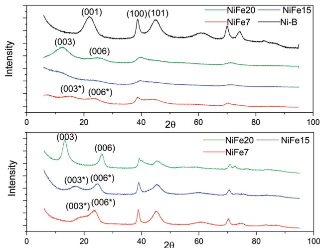
Fig. 2 XRD of Fe doped  $\text{Ni}(\text{OH})_2$  materials. Top: As prepared materials. Bottom: XRD patterns of the iron doped  $\alpha$ - $\text{Ni}(\text{OH})_2$  after 1 month of ageing in KOH (6 M).
