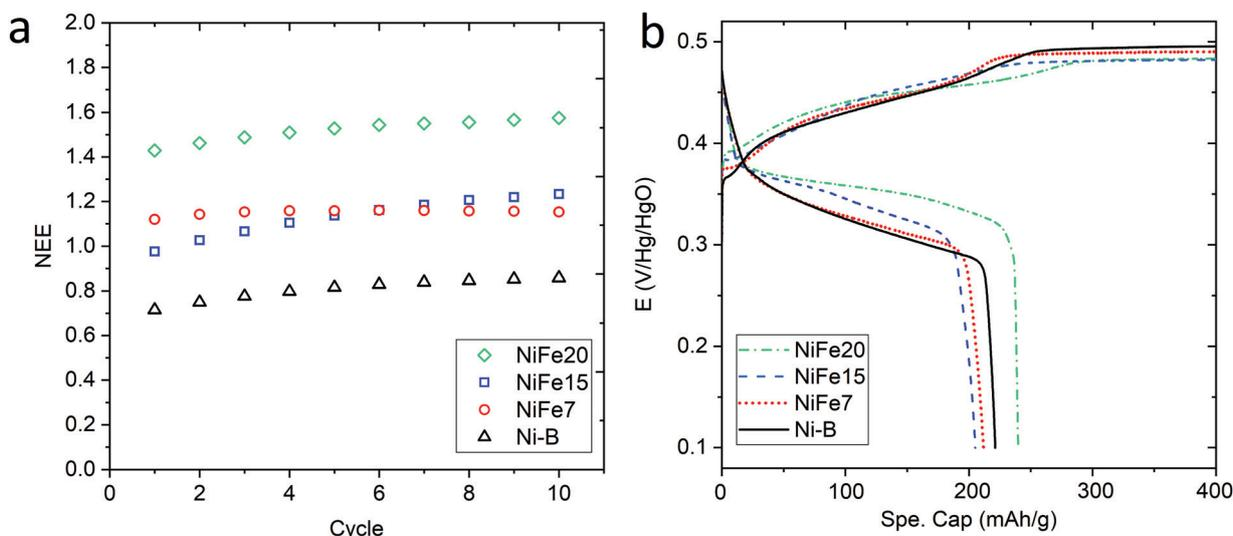
**Fig. 3** (a) Evolution of the NEE per Ni atom through the 10 activation cycles at 0.2C performed on NiFe20 (green diamond), NiFe15 (blue square), and NiFe7 (red circles), compared to  $\beta$ -Ni(OH)<sub>2</sub> Ni-B (black triangle). (b) Charge and discharge curves as a function of the specific capacity (mA h g<sup>-1</sup> of compound) for the 10th activation cycle C-rate = 0.2C.
