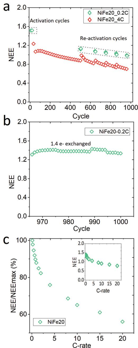
Fig. 5 Characterisation of NiFe2O stability: (a) long-term stability test, (b) after the long-term stability test the electrode is repressed and the capacity of NiFe2O goes back to 1.4e<sup>-</sup> exchanged, and (c) high rate performance of the repressed electrode after the long-term stability test represented by NEE normalised by NEE at 0.1C.
