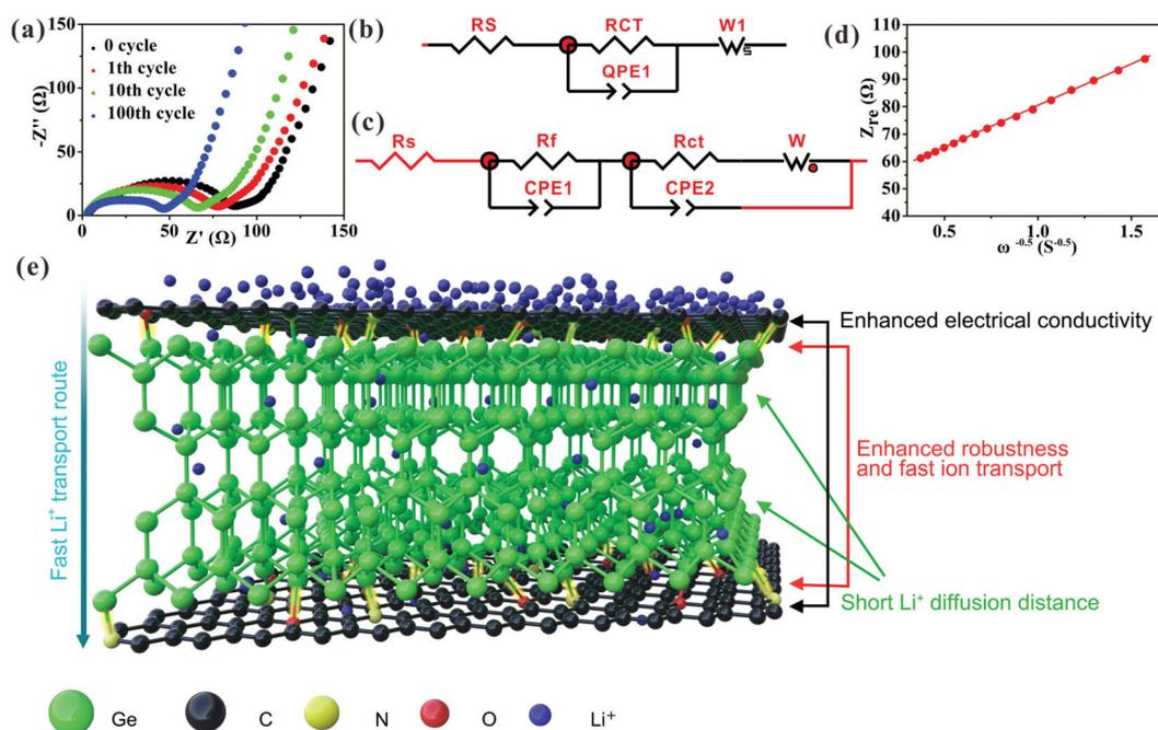
Fig. 4 (a) Nyquist plots before and after cycling, (b and c) Equivalent circuit models before cycling (b) and after cycling (c), (d) Relationship between  $Z_{re}$  with low frequencies after 100 cycles of Ge/C, and (e) Atomic schematic diagram of microstructure of Ge/C.
