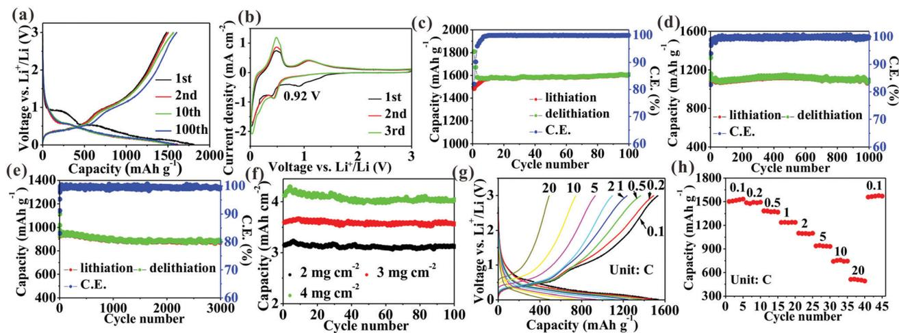
Fig. 3 (a) Voltage profiles at different cycles at 0.1C, (b) CV curves at  $0.1 \text{ mV s}^{-1}$ , (c–e) Cycling curves at 0.1, 2, and 5C, respectively, (f) Cycling curves at different mass loading at 0.1C, (g) voltage profiles at different current densities, and (h) Rate performances of Ge/C. Besides image f, the mass loading is about  $1.1 \text{ mg cm}^{-2}$ .
