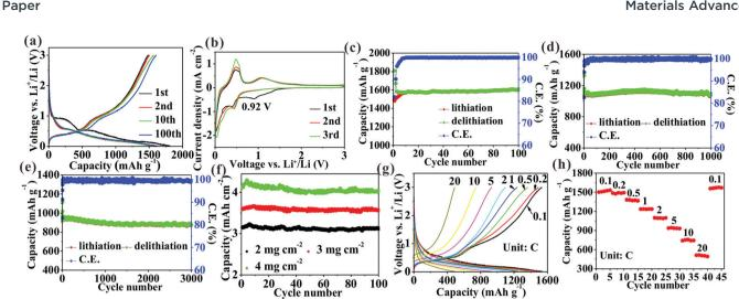
Fig. 3 (a) Voltage profiles at different cycles at 0.1C, (b) CV curves at 0.1 mV s<sup>-1</sup>, (c-e) Cycling curves at 0.1, 2, and 5C, respectively, (f) Cycling curves at different mass loading at 0.1C, (g) voltage profiles at different current densities, and (h) Rate performances of Ge/C. Besides image f, the mass loading is about 1.1 mg cm<sup>-2</sup>.
