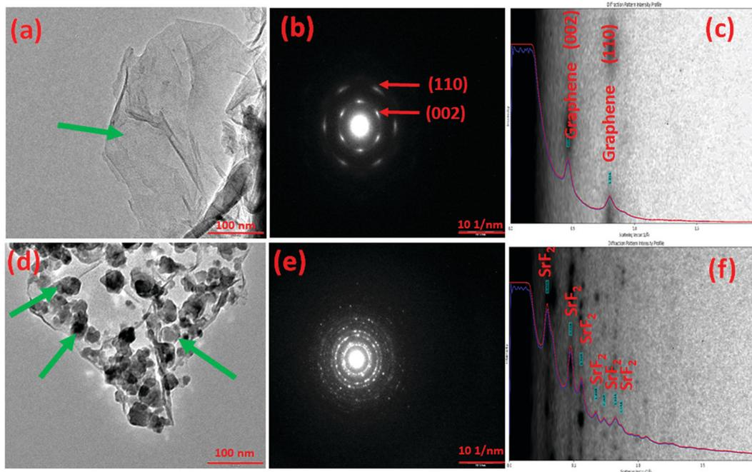
Fig. 1 TEM micrographs of (a) graphene, (b) SAED pattern of graphene, (c) diffraction ring profiler indexing of graphene, (d) SrF<sub>2</sub>@Gr, (e) SAED pattern of SrF<sub>2</sub>@Gr, and (f) diffraction ring profiler indexing of SrF<sub>2</sub>@Gr.
