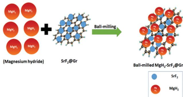
Fig. 2 Schematic diagram for MgH<sub>2</sub> admixed with SrF<sub>2</sub> templated on graphene (MgH<sub>2</sub>-SrF<sub>2</sub>@Gr).
