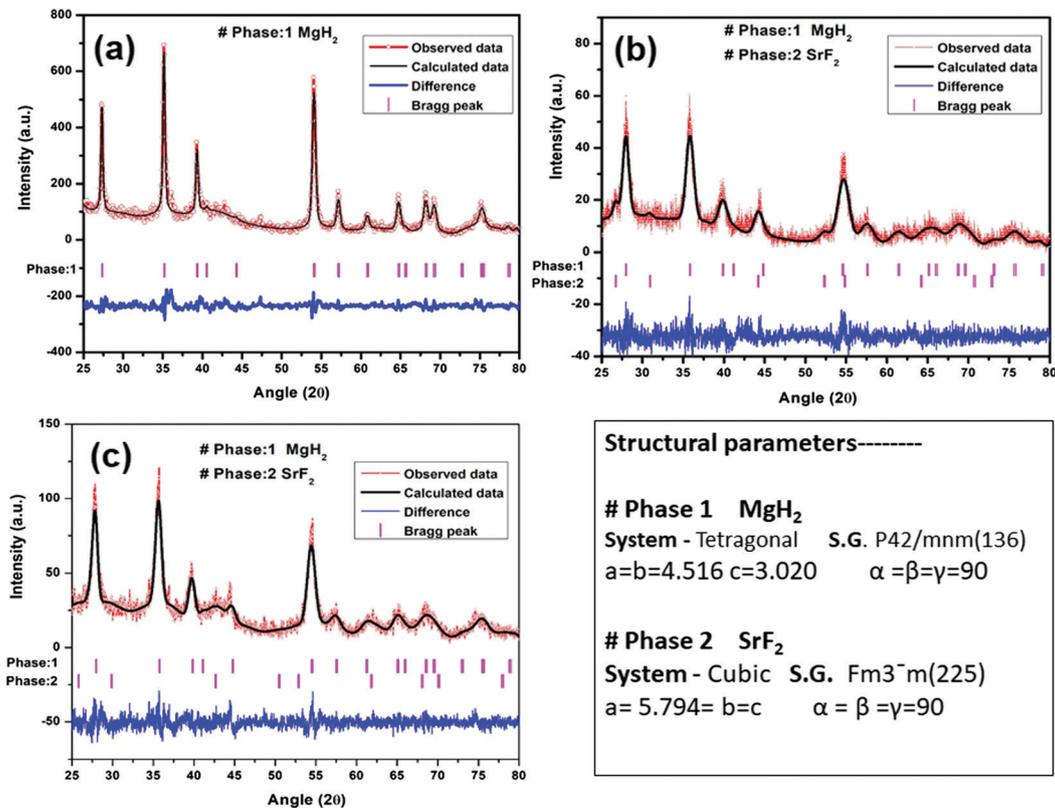
Fig. 3 XRD patterns of  $\text{MgH}_2$  admixed with  $\text{SrF}_2$  and  $\text{SrF}_2$  templated on graphene ( $\text{SrF}_2$ @Gr) with Le Bail fitting using Jana software: (a)  $\text{MgH}_2$ , (b)  $\text{MgH}_2$ - $\text{SrF}_2$ , and (c)  $\text{MgH}_2$ - $\text{SrF}_2$ @Gr.
