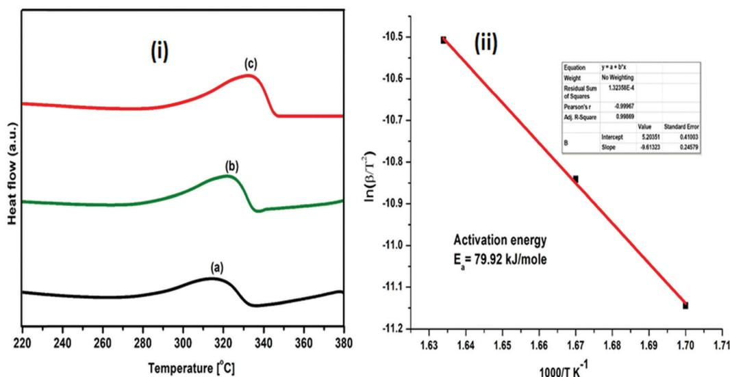
Fig. 10 (i) DSC profiles of  $(\text{MgF}_2 + \text{SrH}_2)@\text{Gr}$  catalyzed  $\text{MgH}_2$  under heating at (a)  $5 \text{ }^\circ\text{C min}^{-1}$ , (b)  $7 \text{ }^\circ\text{C min}^{-1}$  and (c)  $10 \text{ }^\circ\text{C min}^{-1}$ ; (ii) Kissinger plot for evaluating activation energy.
