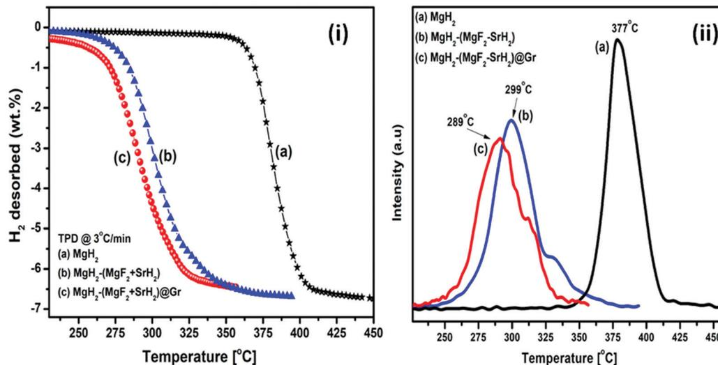
Fig. 6 (i) TPD of  $\text{MgH}_2$  catalyzed by (a)  $\text{MgH}_2$ , (b)  $\text{MgH}_2-(\text{MgF}_2 + \text{SrH}_2)$ , (c)  $\text{MgH}_2-(\text{MgF}_2 + \text{SrH}_2)@\text{Gr}$  and (ii) TPD (peak intensity vs. temperature) of (a)  $\text{MgH}_2$ , (b)  $\text{MgH}_2-(\text{MgF}_2 + \text{SrH}_2)$ , and (c)  $\text{MgH}_2-(\text{MgF}_2 + \text{SrH}_2)@\text{Gr}$ .
