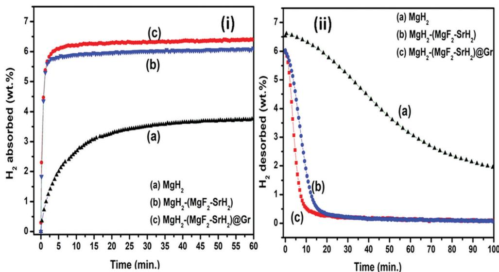
Fig. 7 De/rehydrogenation kinetics profile. (i) Rehydrogenation kinetics curve at 290 °C and 1.8 MPa  $\text{H}_2$  pressure: (a)  $\text{MgH}_2$ , (b)  $\text{MgH}_2-(\text{MgF}_2 + \text{SrH}_2)$ , and (c)  $\text{MgH}_2-(\text{MgF}_2 + \text{SrH}_2)@\text{Gr}$ . (ii) Dehydrogenation kinetics curve at 290 °C and 0.1 MPa  $\text{H}_2$  pressure: (a)  $\text{MgH}_2$ , (b)  $\text{MgH}_2-(\text{MgF}_2 + \text{SrH}_2)$ , and (c)  $\text{MgH}_2-(\text{MgF}_2 + \text{SrH}_2)@\text{Gr}$ .
