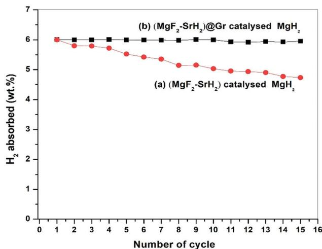
**Fig. 8** Cycling stability up to 15 cycles of (a) (MgF<sub>2</sub> + SrH<sub>2</sub>) catalysed MgH<sub>2</sub> and (b) (MgF<sub>2</sub> + SrH<sub>2</sub>)@Gr catalysed MgH<sub>2</sub>.
