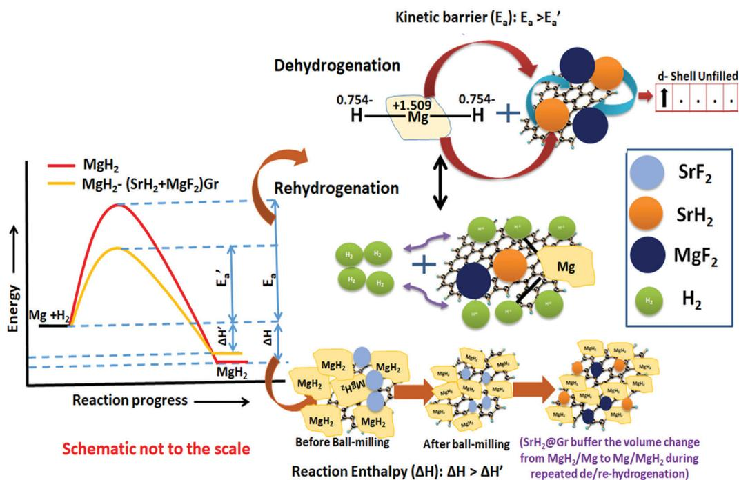
Fig. 13 Schematic diagram of the de/rehydrogenation of MgH<sub>2</sub>–(MgF<sub>2</sub> + SrH<sub>2</sub>)@Gr.
