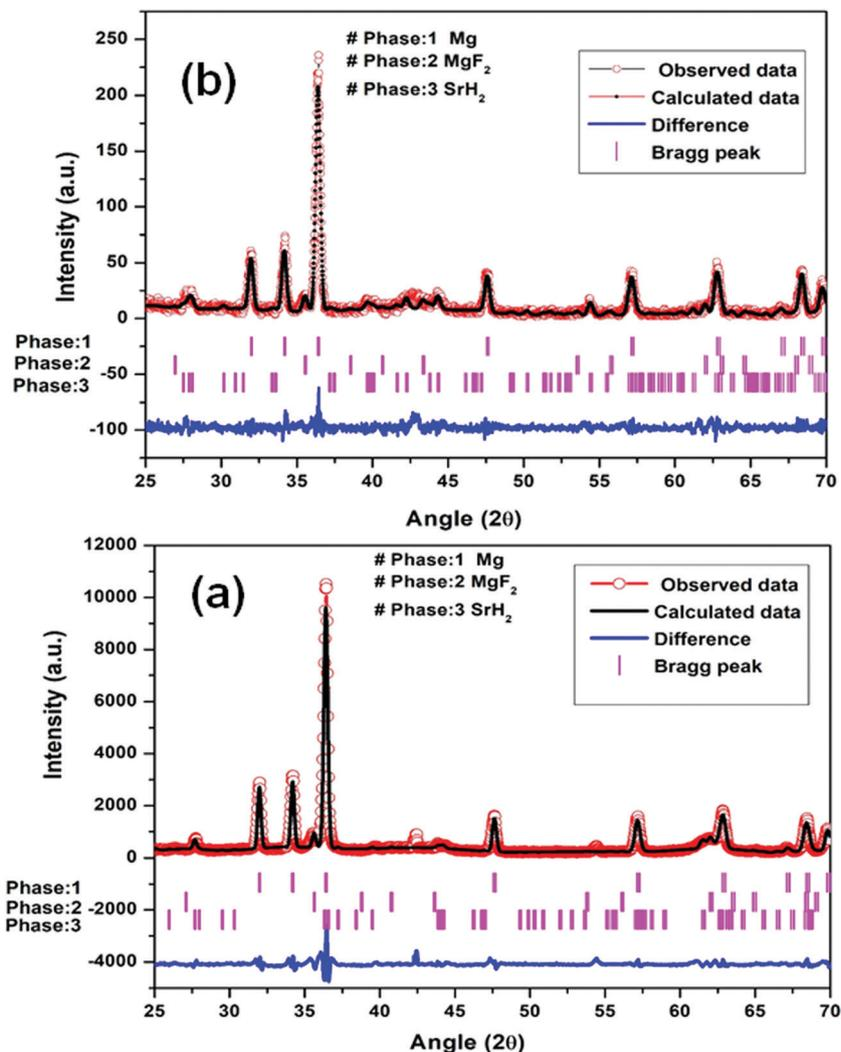
Fig. 5 Le Bail fitting of XRD patterns using JANA software at different steps: (a) Mg-(MgF<sub>2</sub> + SrH<sub>2</sub>) (1st dehydrogenation) and (b) Mg-(MgF<sub>2</sub> + SrH<sub>2</sub>)@Gr (1st dehydrogenation).
