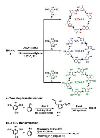
**Fig. 12** Synthetic scheme for RIO COFs (RIO-11, RIO-12 and RIO-13). Two different modulation approaches are shown: (a) two step transimination. (b) *In situ* transimination. Reproduced with permission from ref. 152, Copyright American Chemical Society (2018).
