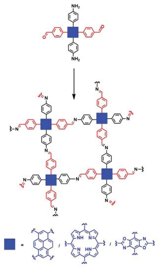
Fig. 31 Schematic representation of COF monomers capable of performing self-condensation. A monomer containing both amine and aldehyde functions is polymerized to an imine COF.
