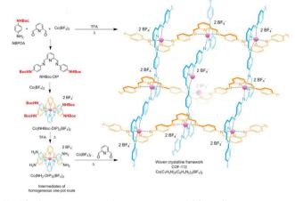
**Fig. 16** Synthetic scheme for the synthesis of COF-112 *via* boc protected amines. Adapted and reproduced with permission from ref. 83, Copyright American Chemical Society (2017).
