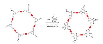
Fig. 26 Schematic representation of the synthesis of  $\beta$ -ketoenamine COF by linker exchange from imine COFs.
