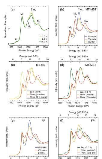
Fig. 3 (a) Deposition time dependence of Al K-edge XANES spectra. (b) Theoretical spectra of w-AIN for the E//a-axis, E//c-axis, and w-AIN powder obtained using MT-MST. Comparison of the theoretical powder and E//c-axis spectra with the experimental spectra of (c) 1.0 h- and (d) 5.0 h-films. (e) Theoretical spectra of w-AlN for the E//a-axis, E//c-axis, and w-AlN powder calculated with FP and (f) comparison with the experimental spectrum of the 5.0 h-film.
