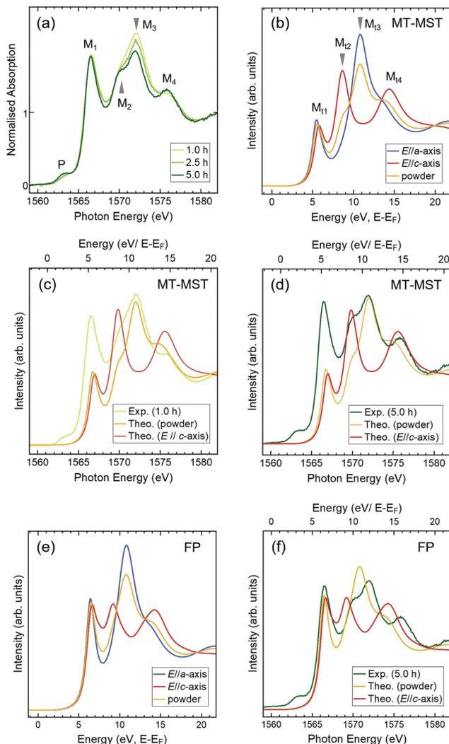
**Fig. 3** (a) Deposition time dependence of Al K-edge XANES spectra. (b) Theoretical spectra of w-AlN for the *E*//*a*-axis, *E*//*c*-axis, and w-AlN powder obtained using MT-MST. Comparison of the theoretical powder and *E*//*c*-axis spectra with the experimental spectra of (c) 1.0 h- and (d) 5.0 h-films. (e) Theoretical spectra of w-AlN for the *E*//*a*-axis, *E*//*c*-axis, and w-AlN powder calculated with FP and (f) comparison with the experimental spectrum of the 5.0 h-film.
