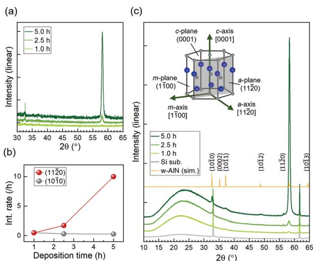
**Fig. 1** (a) XRD profiles of the samples obtained using TF-XRD. (b) Deposition time dependences of (11–20) and (10–10) peak intensities divided by deposition times. (c) XRD profiles of the samples in (a) formed on Si(100) substrates obtained using P-XRD and a simulated powder diffraction profile of wurtzite AlN. Profiles in panels (a) and (c) are shifted in the direction of the longitudinal axis.
