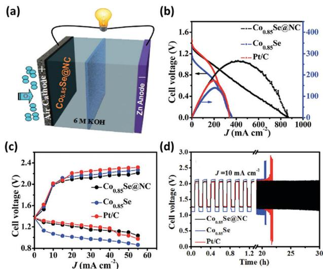
Fig. 14 Electrochemical performance of the  $\text{Co}_{0.85}\text{Se}@NC$  cathode incorporated Zn-air battery: (a) Schematic representation of rechargeable Zn-air battery. (b) Polarization plot ( $V-i$ ) and associated power density plot. (c) Charge/discharge potential ( $V-i$ ) plots. (d) Cyclic stability performance. Reprinted with permission.<sup>25</sup> Copyright 2017 Royal Society of Chemistry.
