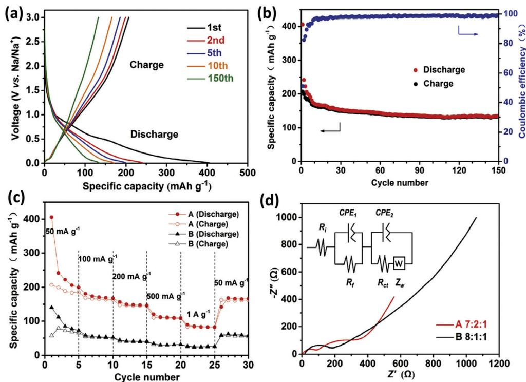
Fig. 8 Electrochemical performance corresponding to  $\text{MgFe}_2\text{O}_4$  micro-box electrodes with varying ratios of the active material, viz., A (7 : 2 : 1) and B (8 : 1 : 1). (a) Discharge–charge potential profiles and (b) cyclic stability performance at  $50 \text{ mA g}^{-1}$  of sample A; (c) rate capability and (d) Nyquist plots corresponding to samples A and B. Reprinted with permission from ref. 9. Copyright 2017 Elsevier.
