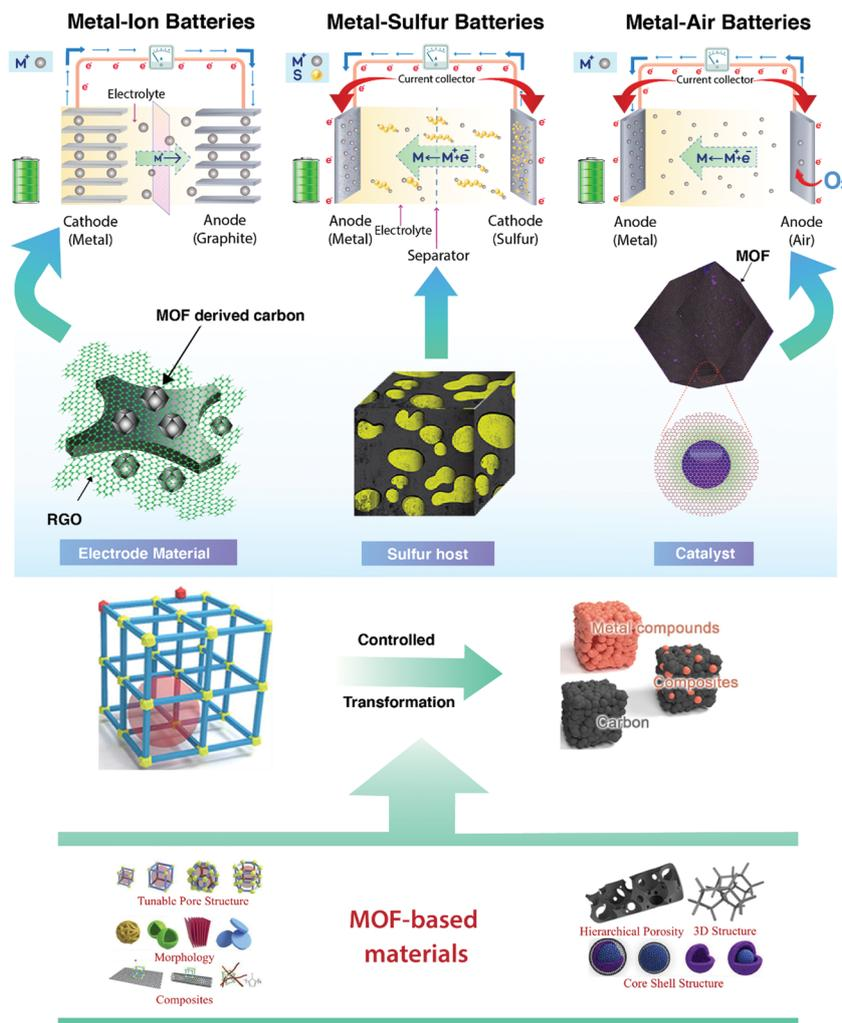
Fig. 1 MOFs in various forms for applications as catalysts, electrode materials, and sulfur hosts in various classes of rechargeable batteries.<sup>25–28</sup> Adapted with permission from ref. 25. Copyright 2017 Royal Society of Chemistry. Adapted with permission from ref. 26. Copyright 2016 Elsevier. Adapted with permission from ref. 28. Copyright 2018 Elsevier.
