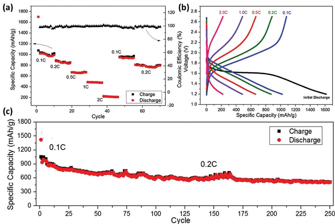
**Fig. 11** (a) C-rate performance exhibited at various current densities by the N-doped carbonized ZIF-8 MOF. (b) Discharge potential profiles at varying C-rates of the Na–S cell with ZIF-8-derived N-doped carbon electrode. (c) Long-term cyclic stability as exhibited by the Na–S cell at 0.1C for the first 5 cycles, followed by 0.2C up to 250 cycles, exhibiting 60% capacity retention after 250 cycles. Reproduced with permission from ref. 112. Copyright 2016 Royal Society of Chemistry.
