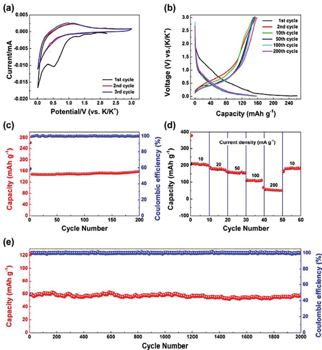
Fig. 6 Electrochemical characteristics of MIL-125 (Ti) MOF as the anode for potassium-ion batteries. (a) Cyclic voltammetry (CV) loops at  $0.5 \text{ mV s}^{-1}$ . (b) Galvanostatic charge-discharge plots at  $50 \text{ mA g}^{-1}$ . (c) Cyclic stability was exhibited at  $50 \text{ mA g}^{-1}$ . (d) Rate performance at various current densities. (e) Long-term cyclic stability at  $200 \text{ mA g}^{-1}$ . Reprinted with permission from ref. 86. Copyright 2017 Royal Society of Chemistry.
