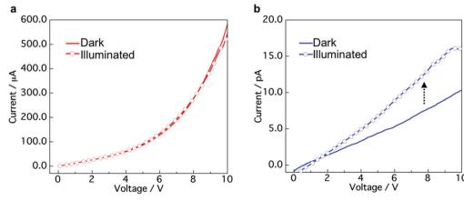
Fig. 6 I-V curves of (a) TTF-TCNQ co-crystals and (b) "phase-separated" crystals in the dark and under white light illumination conditions (9.9 mW cm<sup>-2</sup>).
