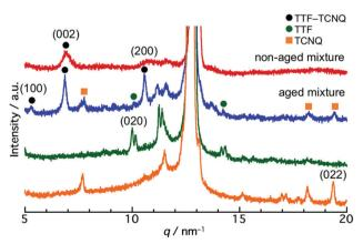
Fig. 3 XRD patterns of the non-aged mixture (red line), aged mixture (blue line), aged TTF crystal (green line), and aged TCNQ crystal (orange line). The diffraction peaks at  $11.5~\mathrm{nm}^{-1}$  and  $12.8~\mathrm{nm}^{-1}$  indicate the diffraction from the filter.
