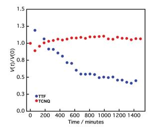
Fig. 4 Normalized crystal size [V(t)/V(0)] vs. time (t) of TTF (blue circle) and TCNQ crystals (red circle) measured by DLS. V(t) is the crystal size at time t, and V(0) is the crystal size at 0 min.
